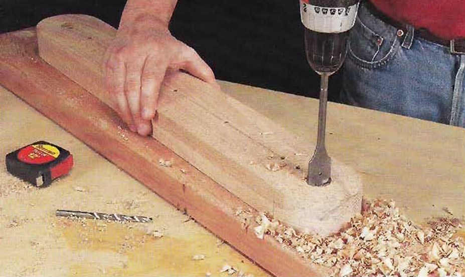
[1] Stick the arms together using double-faced tape, and then drill all the holes. That way, the holes will be aligned in both arms.
