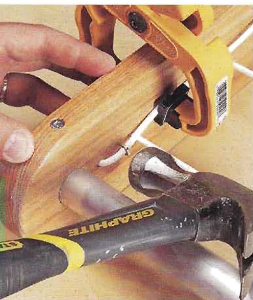
[2] Clamp the clothesline to hold it taut, and then secure it with a \frac{1}{4} " staple.
