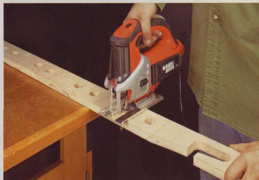
2] Cut the Hook Shapes. Following the layout lines, use a jigsaw to cut the shape of each hook freehand. Then crosscut each hook free from the strip.
