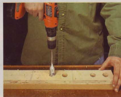
1] Drill the Holes. Use a backer board behind your strip to prevent the holes from blowing out at the back.
