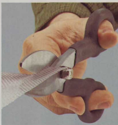
Tin snips or heavy-duty scissors are the best choice for making clean, straight cuts in aluminum screen fabric. The final trim can still be done with a utility knife.
