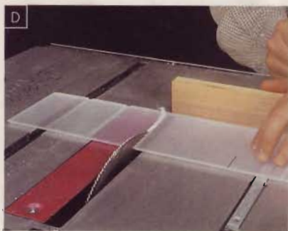
Measure 6\frac{3}{4} " in from each end, and then crosscut the diffuser sides to length. Use a miter-gauge extension for support.
