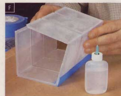
Join the two halves of the diffuser with tape. Flow adhesive onto the mating surfaces and fold the assembly together.
