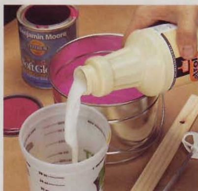
2] Now measure four ounces of a paint conditioner, and add it to the mix. Conditioner helps make the paint cover evenly.
