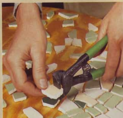
6] As you lay out the design for your tabletop, trim the broken tile pieces to fit using a pair of tile nippers.
