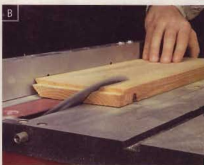
Bevel one edge of each blank. Then reset the rip fence, turn the blank, and bevel rip each one to its final 4" width.
