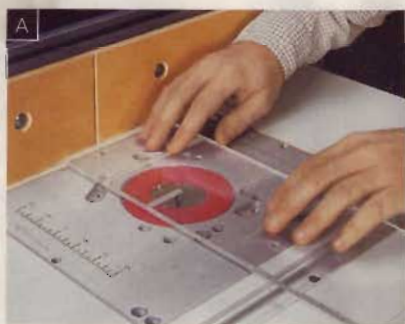
Raise a \frac{1}{4} " straight bit \frac{1}{16} " above the router table, and then rout two grooves near each end of the acrylic blank.
