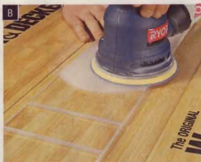
Sand the acrylic using a random-orbit sander equipped with 120-grit sandpaper. Keep sanding until the surface is uniform.
