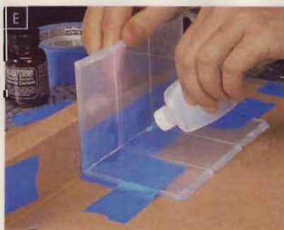
Tape two sides, and fold them to a 90° angle (the table saw fence works great). Then flow acrylic adhesive into the joint.
