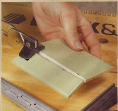
2] Holding the tile tool so that the rubber extensions straddle the scored line, break off the bullnose strip.
