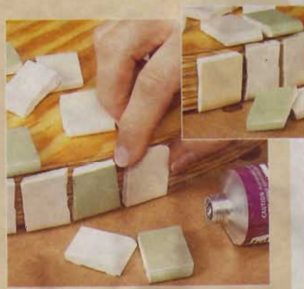
4] Glue on edge tiles so the bullnose is even with the table bottom. On top, it's flush with the face of the edge tiles.
