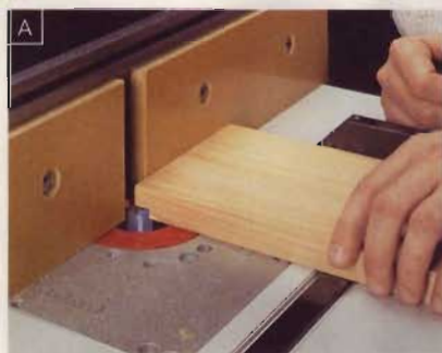
Set up a straight bit to cut a \frac{1}{2}" -wide rabbet \frac{1}{4}" deep. Rabbet one end of the blank, then flip it end-for-end and repeat.
