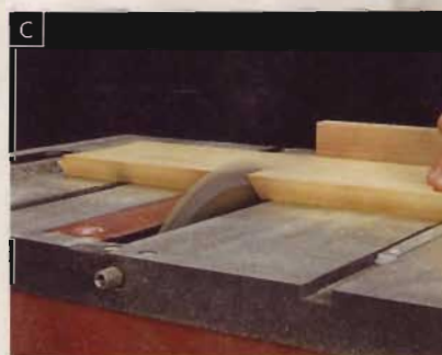
Measure 7\frac{1}{4}" from each end of the blanks, and then crosscut each blank to create two lantern sides.
