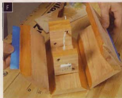
Spread epoxy on the divider edges and on the beveled edges of the sides. Fold the side closed and tape the last corner.
