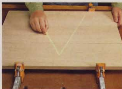
Drawing a large "V" across boards in a panel when test-fitting them makes it easy to reassemble them correctly.
