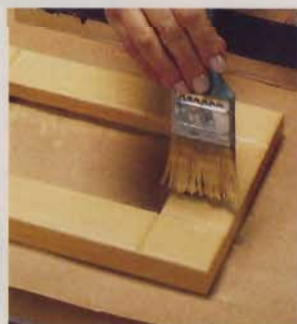
1] Prime and basecoat the frame with a light tan paint to match the topcoat.
