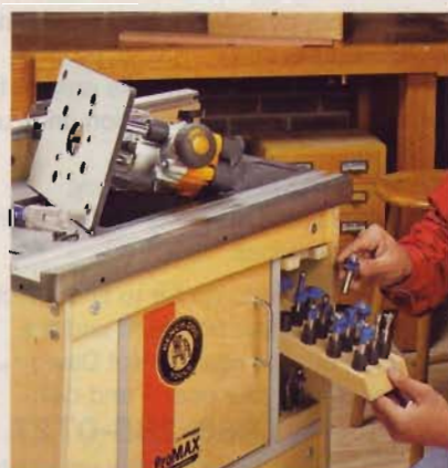
C] Simple slide-out trays made of MDF can be fitted with bit holders or drilled to accommodate a large array of bits.
