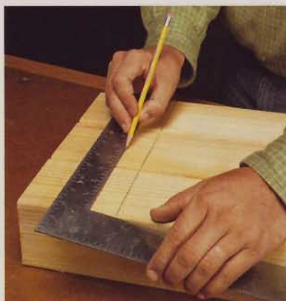
For the best accuracy, hook a framing square over the workpiece. Mark similar parts simultaneously when you can.
