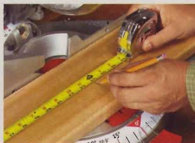
On a miter saw, the blade enters the face of the workpiece. So mark your cutline there for easy blade alignment.
