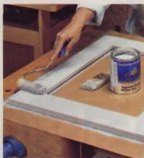
1] Prime and paint the frame with a gray basecoat to complement the metal finish.
