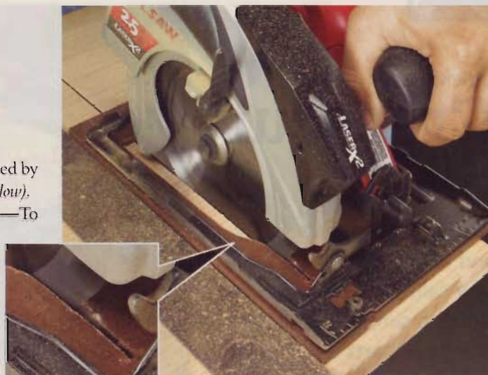
This zero-clearance insert surrounds the blade at the front to prevent the top face of plywood from chipping. The wide notch at the back allows the blade guard to function properly.
