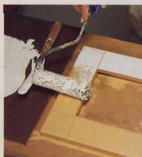
3] Use a 1/2"-nap paint roller to completely coat the face of the frame with compound.
