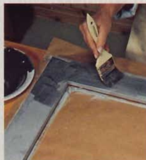
7] Once the paint dries, dab black glaze on the frame with a coarse chip brush.
