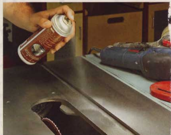
Protect tools during storage by spraying bare metal parts with rust inhibitor.
