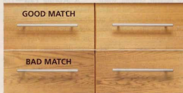
"Flowing" grain makes drawer fronts look great. To get this look, just cut the fronts in sequence from the same panel.
