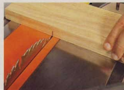
At the table saw, the cutline needs to be marked low on the leading edge, which is where the blade enters.
