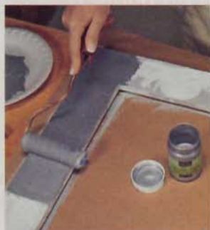
5] When the compound dries, roll the surface of the frame with silver paint.
