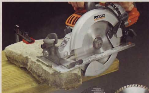
An abrasive or diamond-rimmed blade can turn your circ. saw into a masonry-cutting machine.
