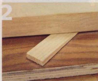
2] Wherever the edges are raised, slip a shim in place. Make sure the shims don't extend past the edges of the sled.
