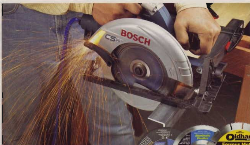
Limited cutting of ferrous and nonferrous metals is possible by teaming a powerful circular saw with a special blade.
