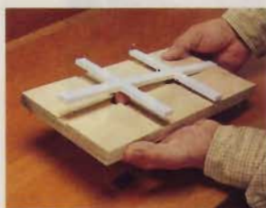
5] Use the holes to pop the muntin bars out of the jig.
