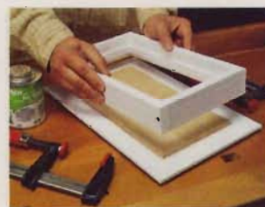
4] Set the trim in the jig, and then glue on the frame.
