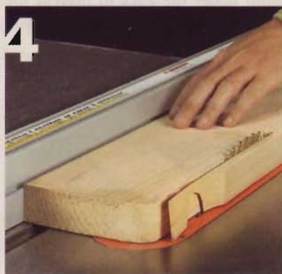
4] Place the jointed edge against the table saw rip fence, and then rip the final edge parallel to the first.
