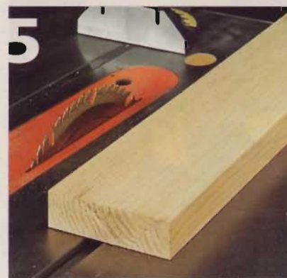
5] To finish dressing your workpiece, crosscut the ends square. Now it's ready to be made into a project part.
