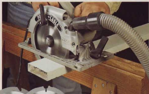
The right blade and a saw with dust extraction reduce the mess of cutting fiber cement.
