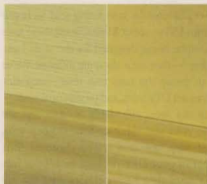
A brushed paint finish makes PVC look like painted wood ( left ). Spray paint gives a glossy appearance ( right ).
