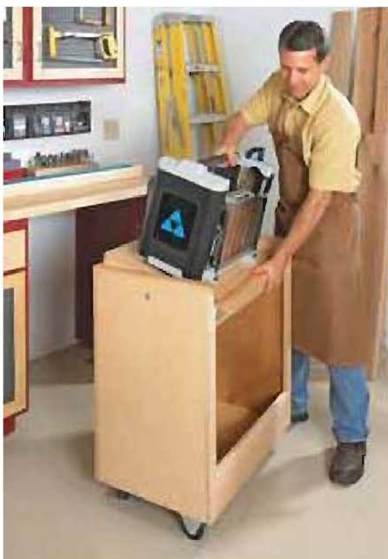
The "flip" top on this cart makes it easy to set up the planer for use (left) or stow it underneath for compact storage (right).
