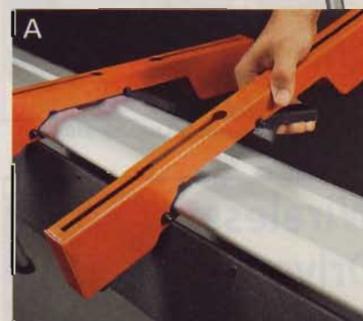
Quick-mount machine supports can accommodate a wide range of benchtop tools.
