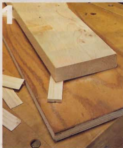
1] Rock the board on the sled until you determine where to place the shims, and then slide them in from the ends.
