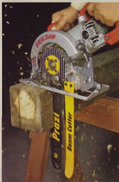
Despite its intimidating appearance, the Prazi Beam Cutter cuts smoothly and with little user effort.
