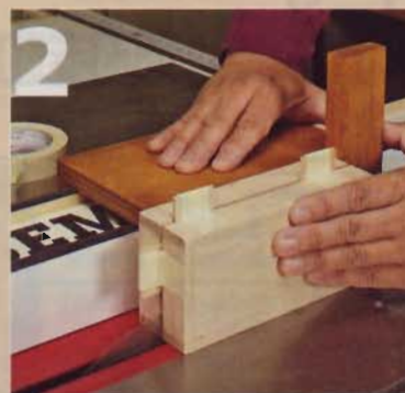
2] Shims taped into the saw kerfs prevent the box parts from binding against the blade on the final pass.
