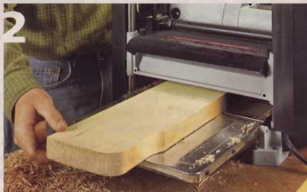
2] Place the jointed face against the planer table, and plane until the second face is flat and parallel with the first.
