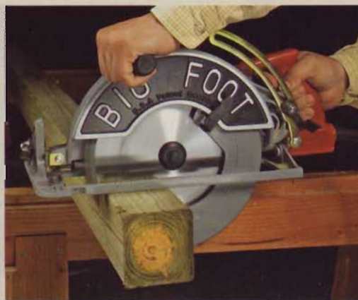
The Big Foot kit was invented by a carpenter who wanted a saw capable of cutting two 2x4s at one time. It's also great for 4" posts.
