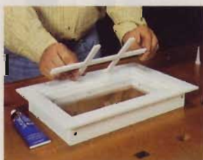
6] Attach the muntin bars to the glass with silicone.
