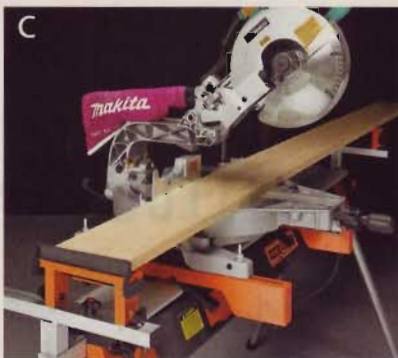
Breaking down long workpieces is much simpler with the expandable stock supports and built-in flip stop.
