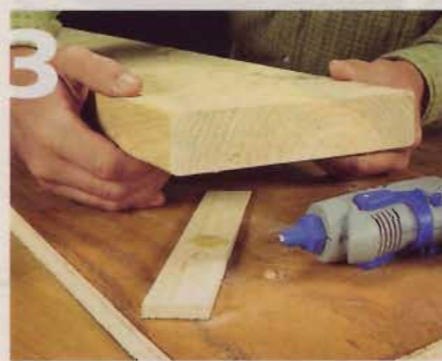
3] Use hot glue to hold the shims to the sled, and then stick the board to the shims the same way.
