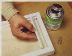
2] Set the glass stops on the jig, and glue them in place.
