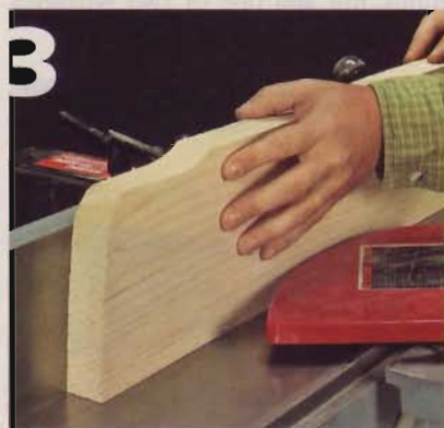
3] Use the jointer to straighten one edge of the workpiece. Press one face against the fence to ensure a square corner.
