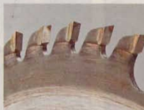
Resin buildup on a saw blade reduces blade life.
