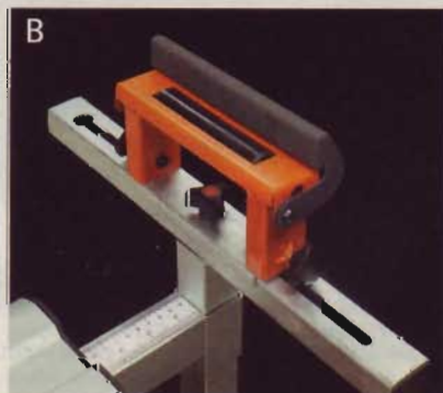
The stock support extends for long workpieces and can be adjusted to match various tool heights.
