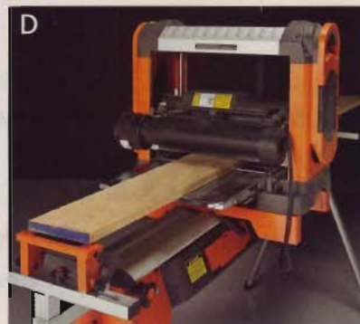
Rollers on the stock supports make them perfect for infeed and outfeed support for a thickness planer.
