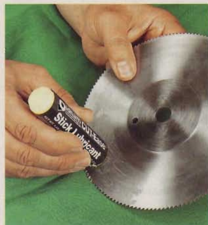
Use the blade lubricant like a crayon, and "color" the entire blade to help it cut more efficiently.
