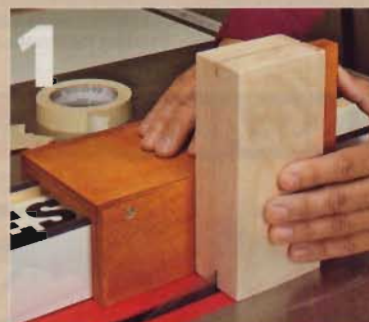
1] Hold the box firmly against the jig as you cut the ends. Keep the same face against the jig for both cuts.
