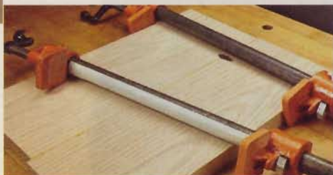
A strip of tape makes a quick clamp cover to prevent stains during glue-ups.
