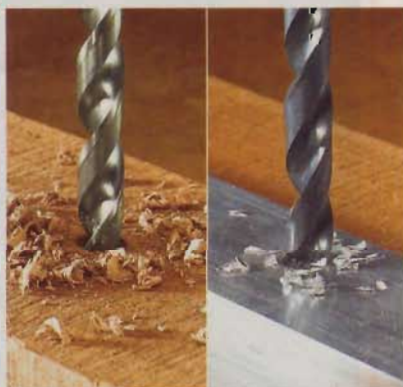
Tightly fluted bits drill quickly in wood ( left ), but they “grab” in metal, so use standard-flute bits instead ( right ).
