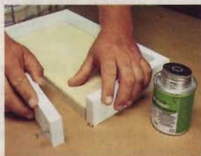
1] Glue and screw the frame pieces around the jig.
