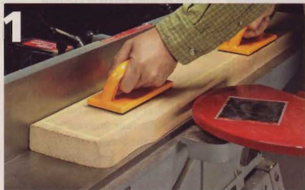
1] Joint the first face by making multiple shallow passes (removing no more than \frac{1}{32} " per pass) until the face is flat.
