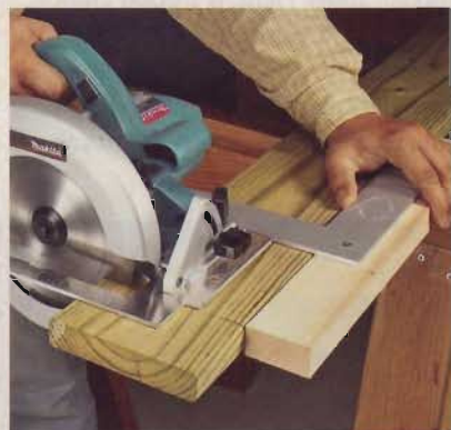
The end of the auxiliary fence on this ChopShot guide makes aligning the blade with the cutline simple.
