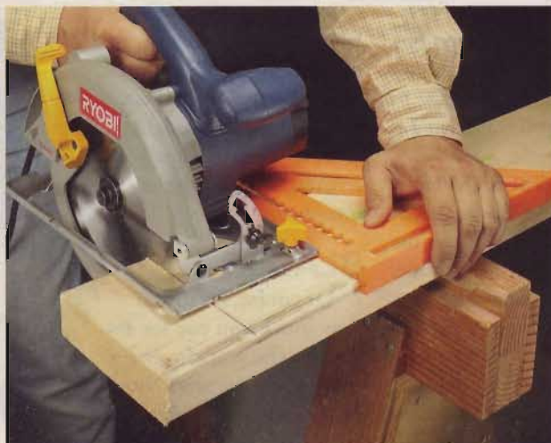
A common speed square can serve as a quick and effective cutting guide when working with lumber as wide as 6". You can simply hold it with your free hand or clamp it for a more secure guide.
