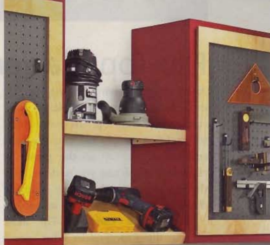
The upper shelves can be mounted level (with the front edging facing down) or at an angle (edging up).
