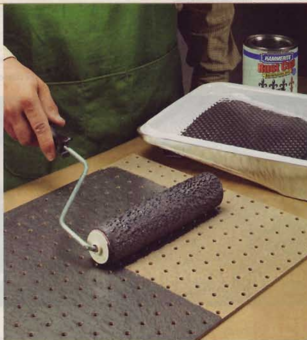
This Hammerite paint gives shop projects the interesting look of "hammered" metal. Sanding the surface lightly and then using a mohair roller yields the best results.
