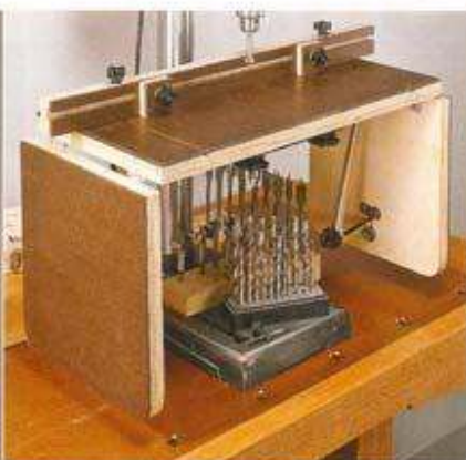
Even with the leaves folded down, this drill-press table offers two square feet of workspace.
