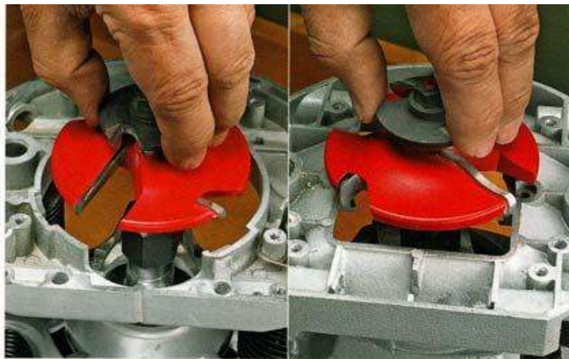
Bosch's large base opening ( left ) easily accommodates a 3½" panel-raising bit. The much smaller opening on the Freud ( right ) makes using bits this large difficult.
