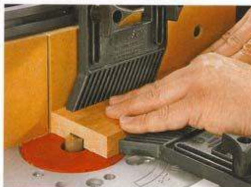
ROUTING THE FACE. By positioning the fence away from the bit, you can rout the face of a workpiece ( Photo, left ). If you need to widen the cut, move the fence farther away from the bit before making a second pass ( Illustration, right ).
