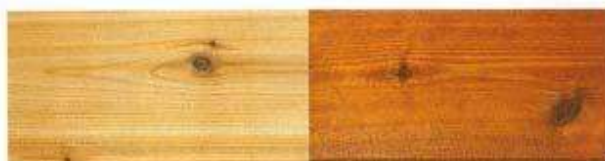
Clear stains (left) have trans-oxides that filter the sun's UV rays. Semi-transparent stains (right) use pigments to block the rays.
