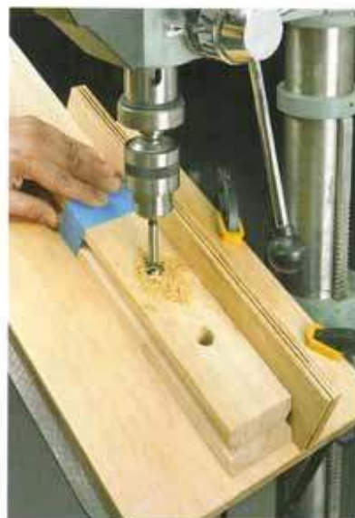
To drill evenly spaced, angled holes in the keeper strips for the balusters, I used this drill press jig (see page 88).
