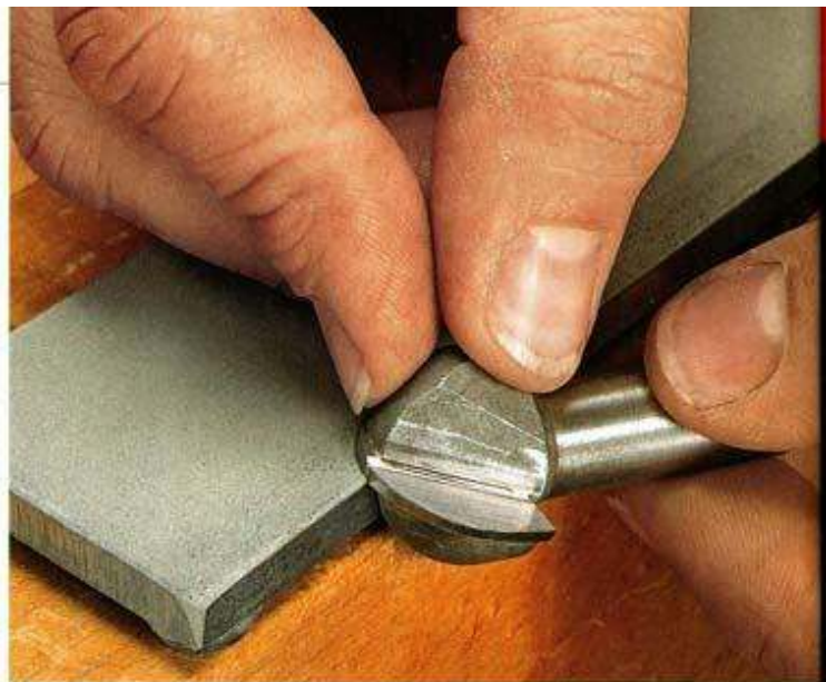
A few passes over a diamond sharpening stone will maintain a sharp cutting edge on most types of router bits. Hold the bit flat against the stone for a consistent edge.
