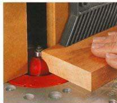
Piloted Bits. The fence can enhance control with piloted bits. Set the fence so the bearing just clears the face (below).
