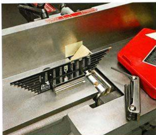
A powerful magnet holds the Blade Gauge III on the jointer outfeed table. As soon as the knives contact the metal gauge, it completes a circuit and illuminates a small light.
