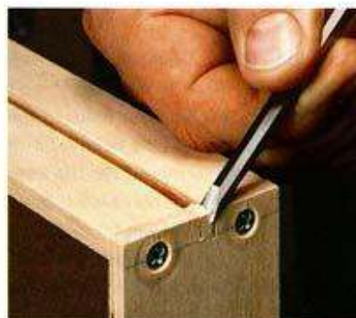
Extend the groove through the drawer back by cutting and chiseling a small notch in the back.
