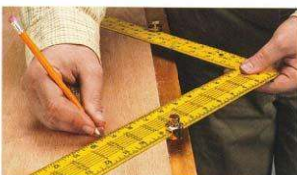
By attaching the gauges to both legs of the square and then placing the square so the legs extend out over a workpiece, you can mark an angled line across the piece.
