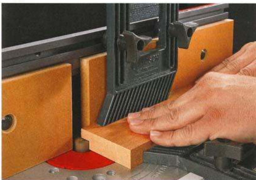
ON THE EDGE. By changing the position of the router-table fence, you control how much of the bit is exposed and, in turn, how wide of a cut the bit makes.
