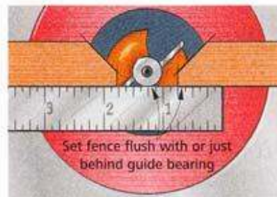
Piloted Bits. The fence can enhance control with piloted bits. Set the fence so the bearing just clears the face (below).
