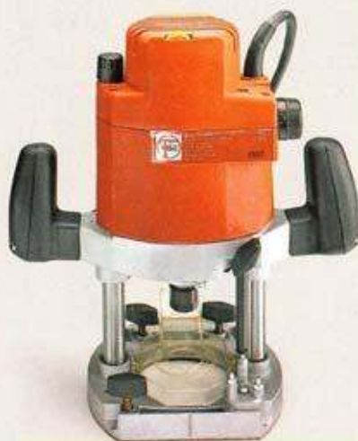
Five fixed positions on the Bosch turret ( above ) make it easier to rout a series of progressively deeper passes than turrets with just three adjustable positions ( Inset ).
