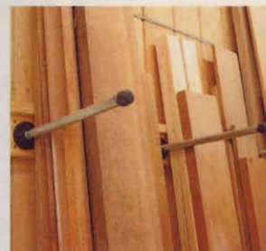
Pipe and plumbing fittings make a simple lumber rack.
