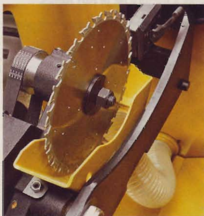
The shroud and dust hose inside the PM2000 capture dust at the source and direct it straight to the port.
