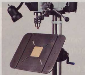
The Delta's large table tilts 45° forward, as well as 90° to either side.
