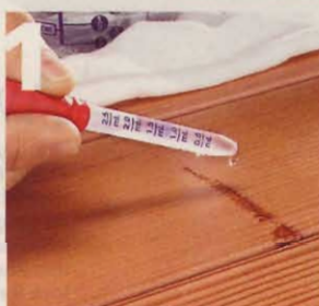
1] Use an eye dropper to saturate the dent with water.
