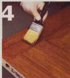
4] After staining one side of the door, use a "dry brush" to brush with the grain until the stain is smooth and even.
