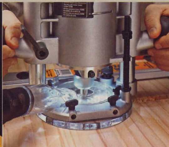
High-output L.E.D. lights in the motor housing of the Ridgid R2930 router offer a better view of the bit. A dust-collection port is included for both the plunge and fixed bases.
