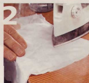
2] Apply an iron to a damp cloth to steam out the dent.
