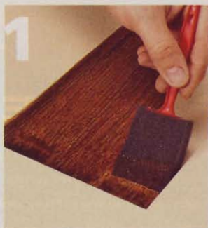
1] Starting with the panels, use a foam brush to apply stain. Choose a thick, heavily pigmented stain (like Zar).
