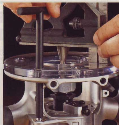
A T-wrench for making through-the-table adjustments is also handy for fine-tuning handheld setups.
