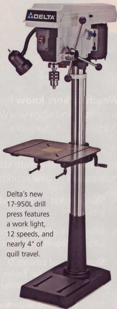
The Delta's large table tilts 45° forward, as well as 90° to either side.
