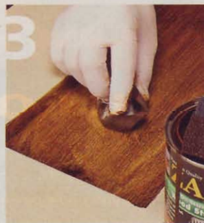
3] Now apply light to medium pressure as you remove the excess stain. Wipe the rag back and forth with the grain.
