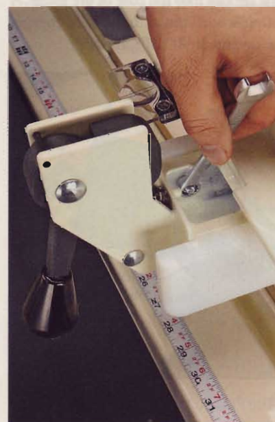
By loosening screws inside the body of the fence, the faces on the Jet fence can be adjusted for clearance.
