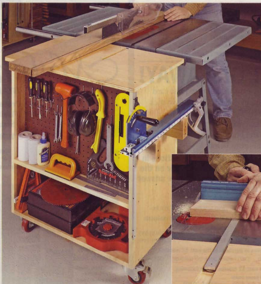
When ripping long boards, the top of this cart provides sturdy outfeed support. Clearance slots for the bar on the miter gauge let you crosscut, as well ( Inset ).
