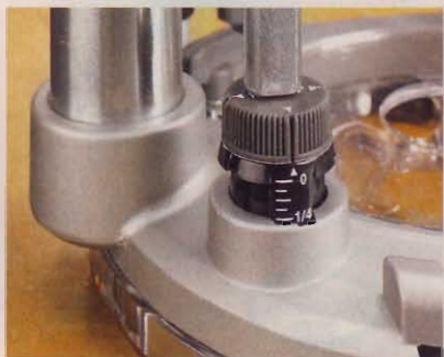
Use the depth stop rod to get close, and then make the final adjustments using the adjustable stop.
