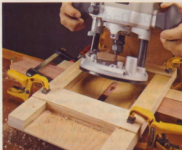
This simple jig works with a plunge router to make keyhole slots. It also can be used to make other stopped slots, grooves, or dadoes in a workpiece.
