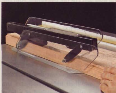
A two-piece blade guard on the PM2000 keeps the blade covered when ripping thin pieces.
