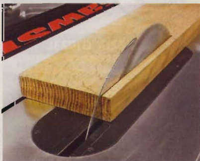
SawStop's riving knife moves with the blade, prevents binding, and can be used when conventional splitters can't.
