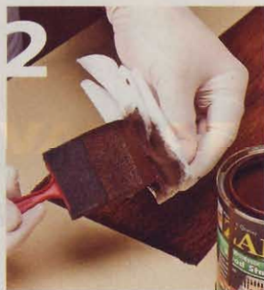
2] Before you remove excess stain, dab a rag with the stain. This prevents the rag from removing too much stain.
