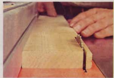
3] To complete the seat edging, move to the table saw and rip the rounded edge free of the board.
