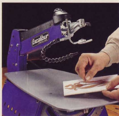
Pierce cuts are simple with the arm lifted out of the way and the blade secure in the lower clamp.
