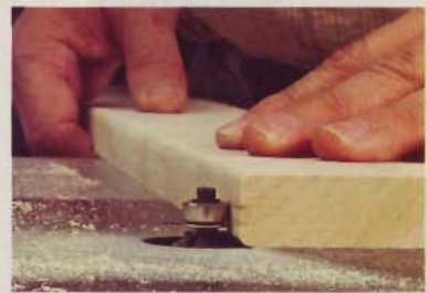
2] Flip the board end-for-end, and round over the second edge using the same router-table setup.
