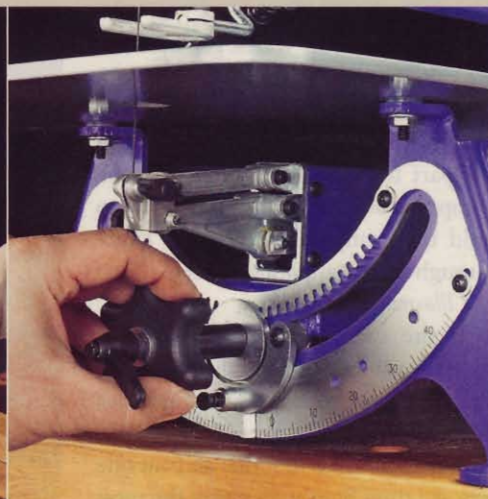
A large adjustment knob and two drive gears (front shown) make adjustments smooth. A locking lever holds the arm at the desired angle.
