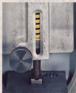
1] The "detension" setting takes pressure off the blade when it's not in use.
