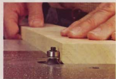
1] After ripping one edge of a long board straight, rout a \frac{1}{8} " roundover along the edge.
