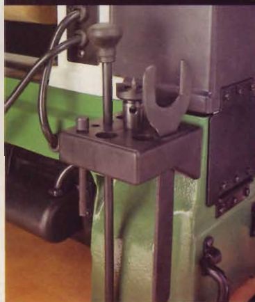
A 12-position indexing head and an accessory tray are Rikon extras not found on competitive lathes.
