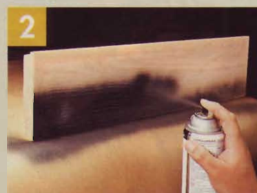
▲ Hold the can perpendicular to the wood, and spray on 2 to 4 coats until the pores are filled.
