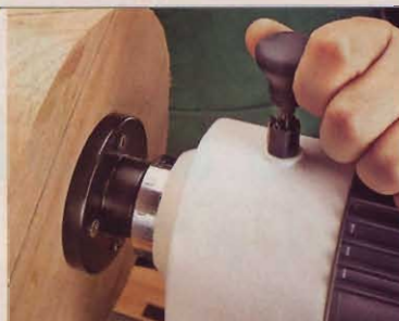
A 12-position indexing head and an accessory tray are Rikon extras not found on competitive lathes.
