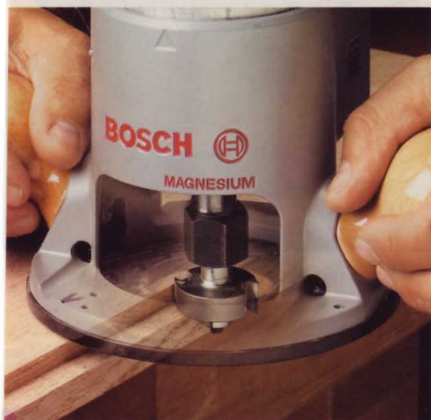
A SHOULDER TO LEAN ON A rabbeting bit cuts a right-angle profile. This seemingly simple cut can be used to produce versatile joinery.
