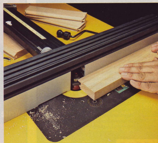
◀ By using the SmartLift Digital's "zero" feature and recording the height of each setup as it appears in the digital display, elaborate projects such as this raised-panel door can be easily repeated.
