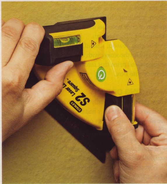
▲ The Stanley S2 Laser Square must be held level as you mount it because there is no way to adjust the line once the level is secured to the wall.
