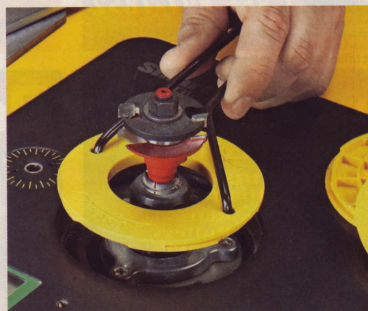
▲ With the SmartLift raised to its maximum height, the collet nuts are easily accessible for above-the-table bit changes.
