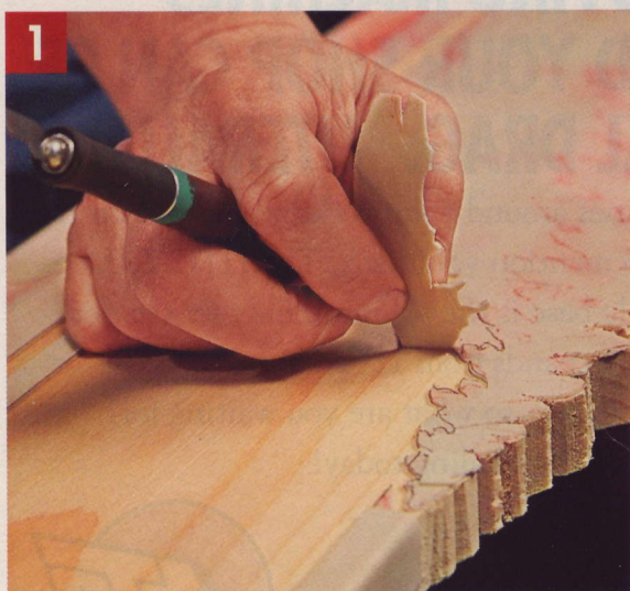
▲ After cutting around the “resist,” the areas to be sandblasted are peeled away to reveal the bare wood. Any cutouts are made with a jig saw or scroll saw.
