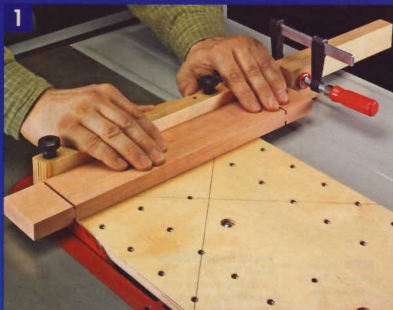
▲ Align the shoulder location with the edge of the sled, and make passes, flipping the piece in between. A stop block speeds setups.
