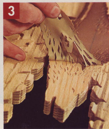
▲ After blasting, the resist is carefully peeled away to reveal the raised, smooth areas.
