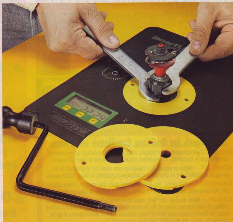
▲ With the SmartLift raised to its maximum height, the collet nuts are easily accessible for above-the-table bit changes.
