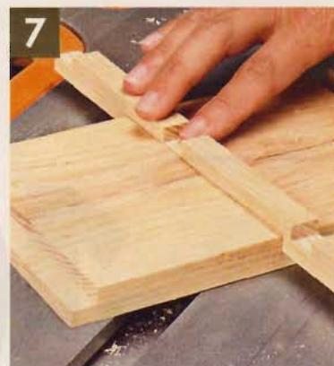
▲ CHECK THE FIT. Once you're satisfied with the fit, rip the remaining strips from the blank.
