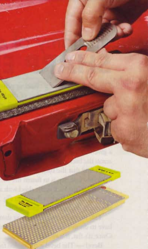
▲ These double-sided diamond stones from Eze-Lap ( top ) and DMT ( bottom ) have a different grit on each face for more versatility.
