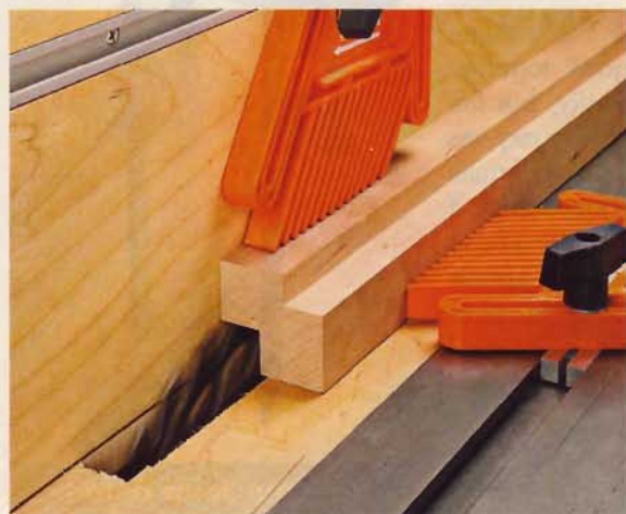
▲ Use an auxiliary fence butted against a \frac{3}{4} " dado blade while rabbeting the edging. Cut one rabbet with the blade raised to \frac{1}{2} ", and the other at \frac{3}{4} ".
