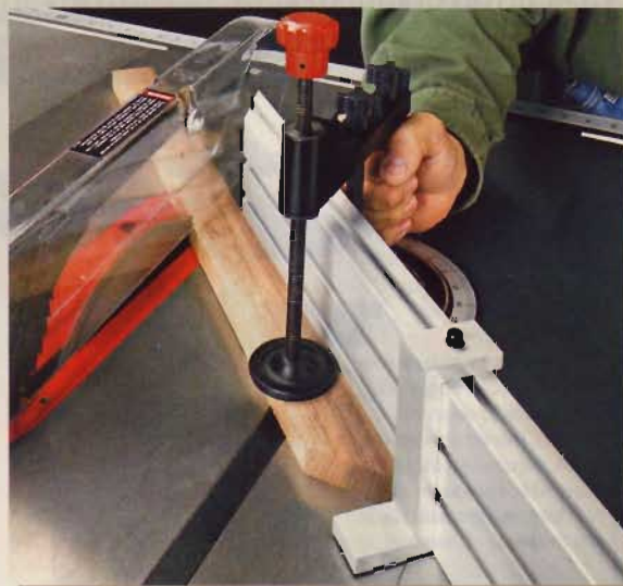
▲ Each miter gauge was checked for play in the miter slot and for general quality.
