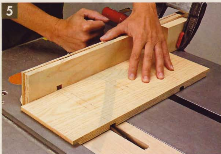
▲ DEAD-ON DADOES. After laying out the locations of the dados on an extra-wide blank, align the marks with the notch in the miter gauge fence. Then clamp a stop block to the fence and make the cut.
