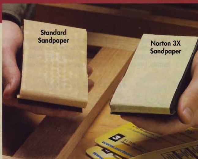
▲ As a test, I made 200 passes with both 3X sandpaper and standard sandpaper. The standard paper was worn smooth, with almost no grit ( left ). The 3X looked good as new ( right ).
