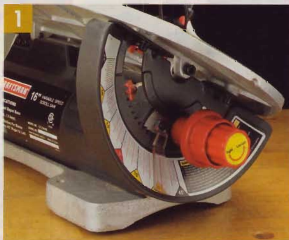
▲ A two-stage dial adjusts and locks the bevel of the table. A large, easy-to-read scale and detents make accurate setup effortless.
