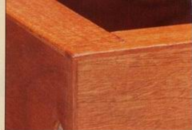
▲ The thin strips of wood covering the exposed plywood edges of the drawers make the joint lines virtually disappear.
