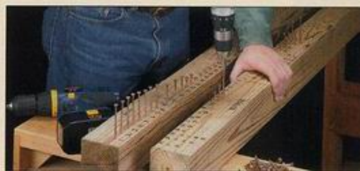
▲ We compared the clutches on the drills by driving a screw at each setting.
