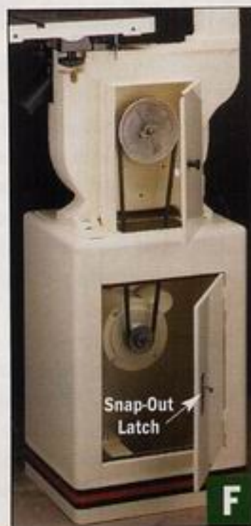
▶ The Jet makes it easy to service the entire saw by hinging every cabinet door.
