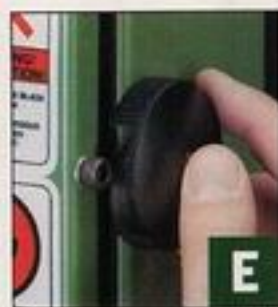
▲ Threaded knobs like those on the Powermatic make it inconvenient to open the wheel covers.
