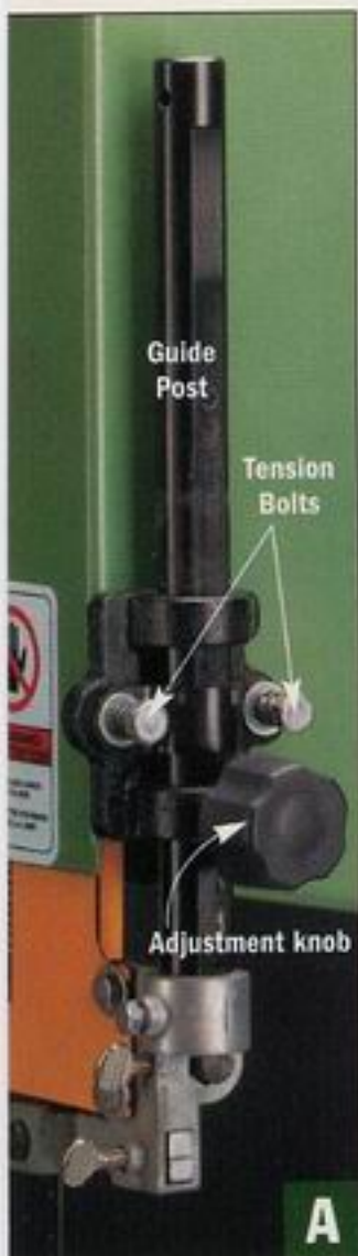
▲ General's tensioned guidepost operates smoothly.
