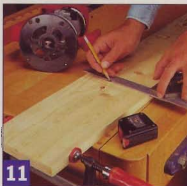
You can save time and reduce mistakes if you mark identical parts, like these ladder uprights, simultaneously.
