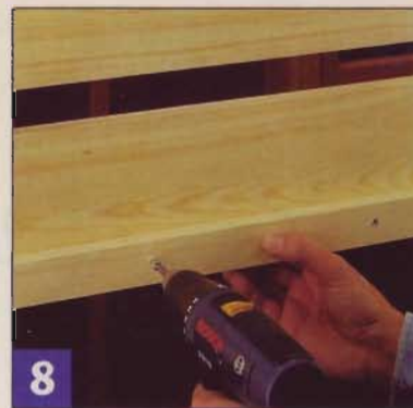
Fasten 1x2 cleats to the inside faces of the platform rails. These support the plywood panel for the mattress.
