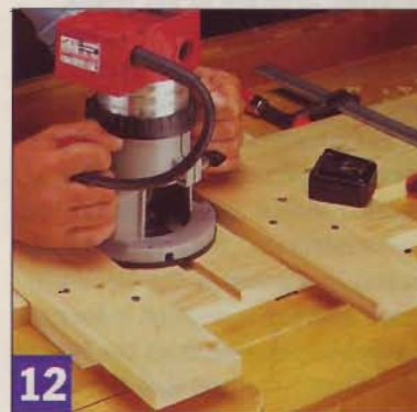
With the ladder uprights still clamped together, align the dado jig with layout marks on the workpiece, then rout.
