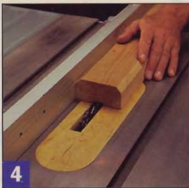
4 Plough a \frac{3}{4} " x \frac{3}{16} " groove in the bottom of the caps. Lower the blade \frac{1}{16} " and groove the screen caps' top face.
