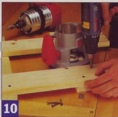
Use your router base to check the spacing of the guide rails on the dado jig. Then recheck square and fasten.
