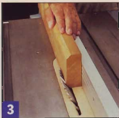
3 Tilt the table saw blade to 45° and cut a \frac{3}{8} " chamfer on the top corners of all the 2x4 screen and top caps.
