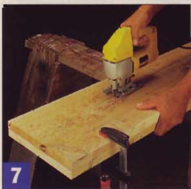
7 With the curve laid out, clamp the arched rail stock together and cut the curve with a jig saw. File and sand the edges smooth.
