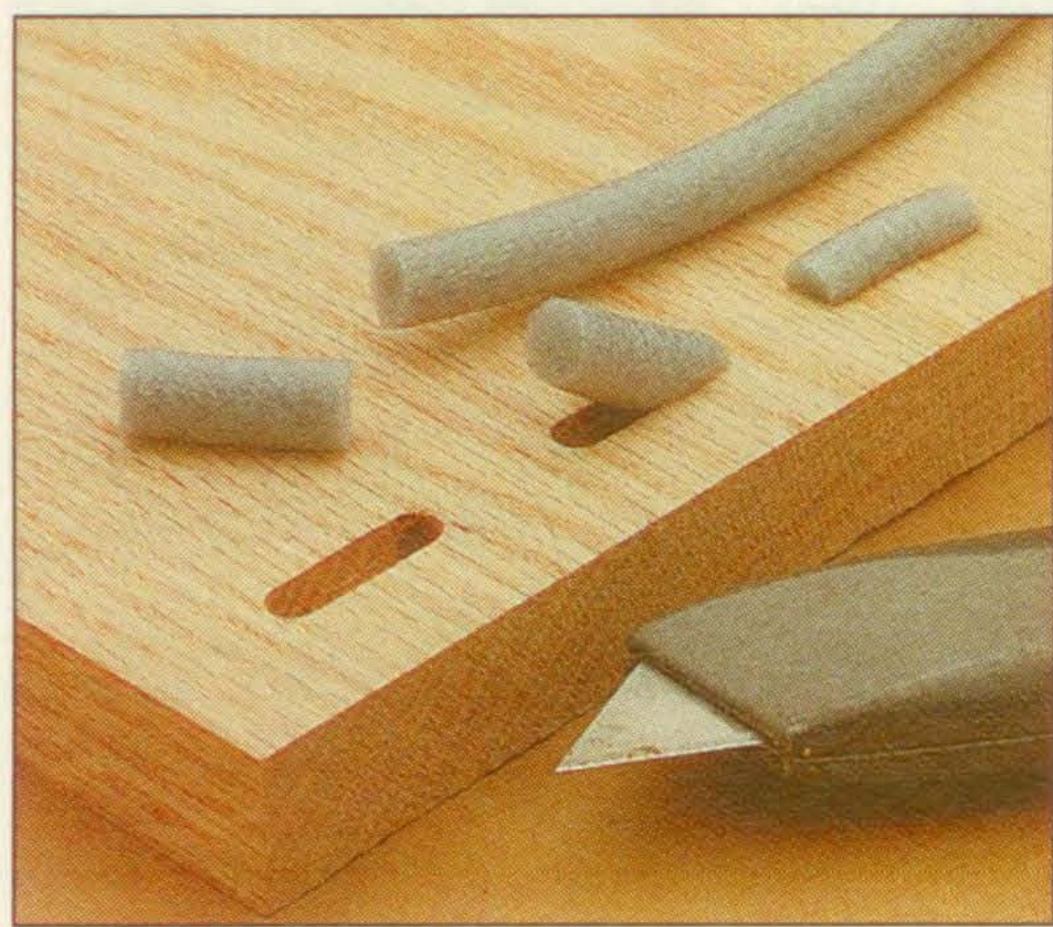
▲ Plug the Mortise. A short strip of foam caulking rod does a great job of keeping finish out of the mortise before glue up.
