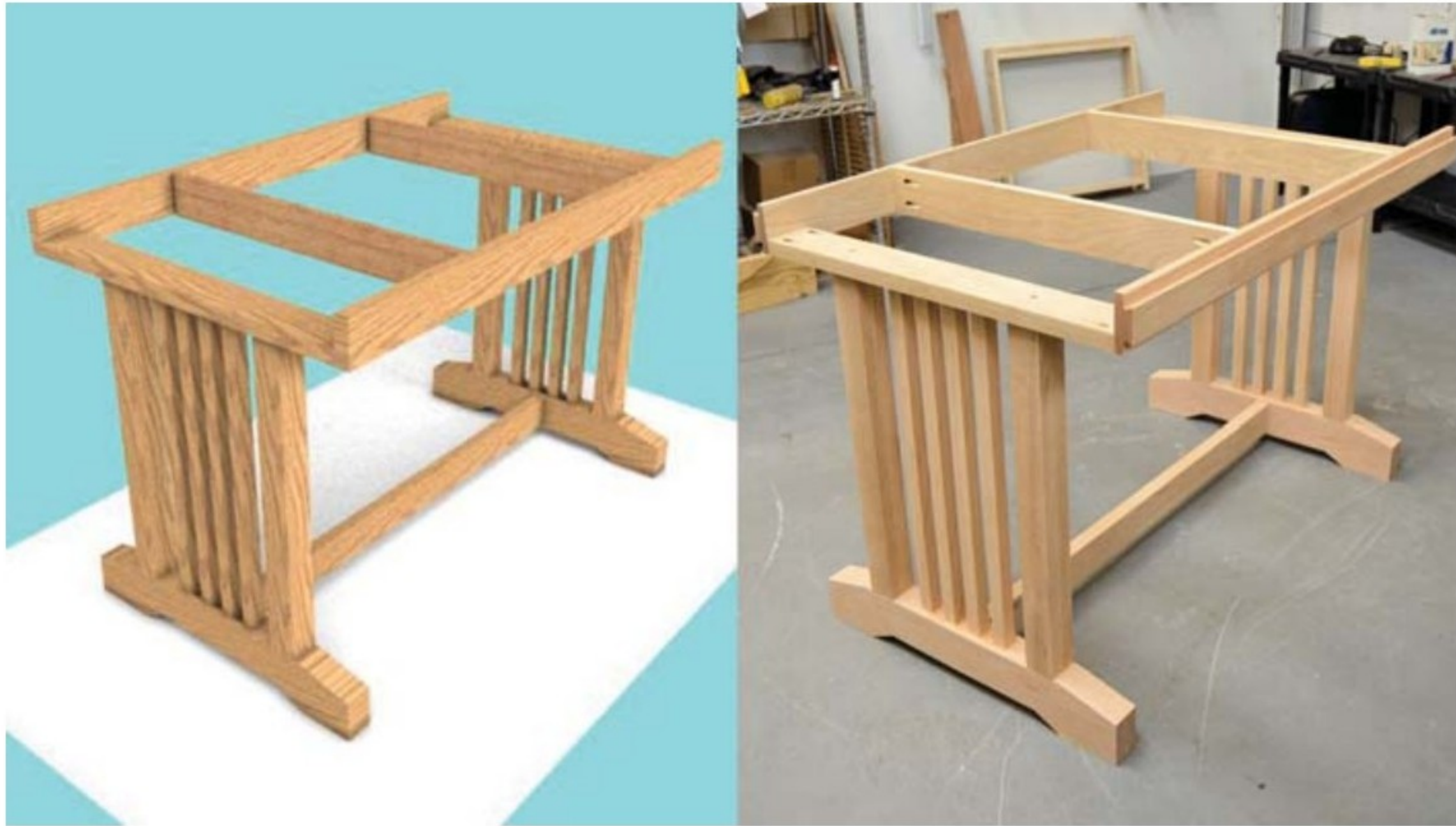
Sketchlist assembly of a table trestle beside a photo of the actual parts.
