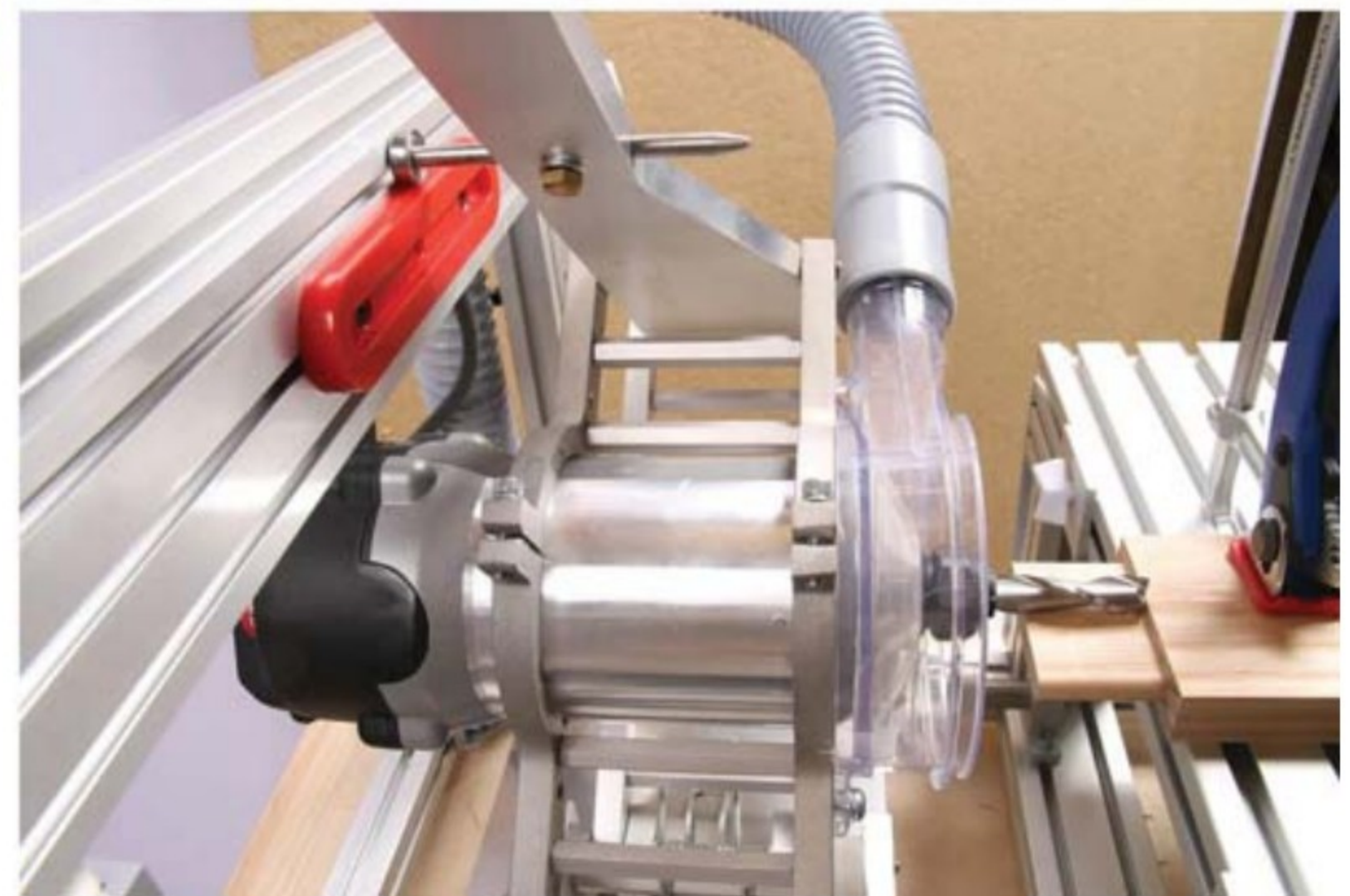
Equipped here with a Bosch motor, the PantoRouter is a user-friendly solution for high quality, precise joinery in solid wood.
