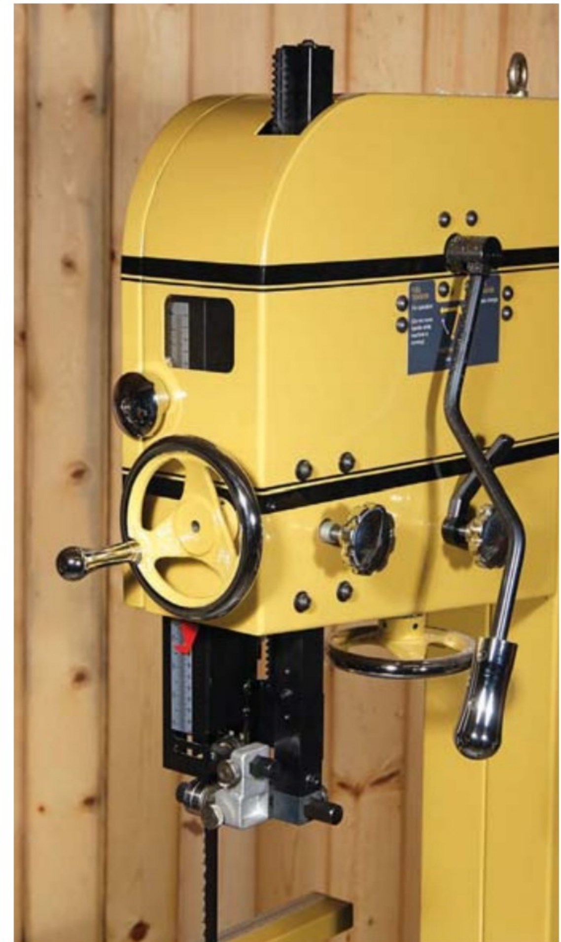
Powermatic's PM1500 combines a 3-hp motor with cast-iron wheels and a heavy table to deliver smooth, vibration-controlled cutting.
