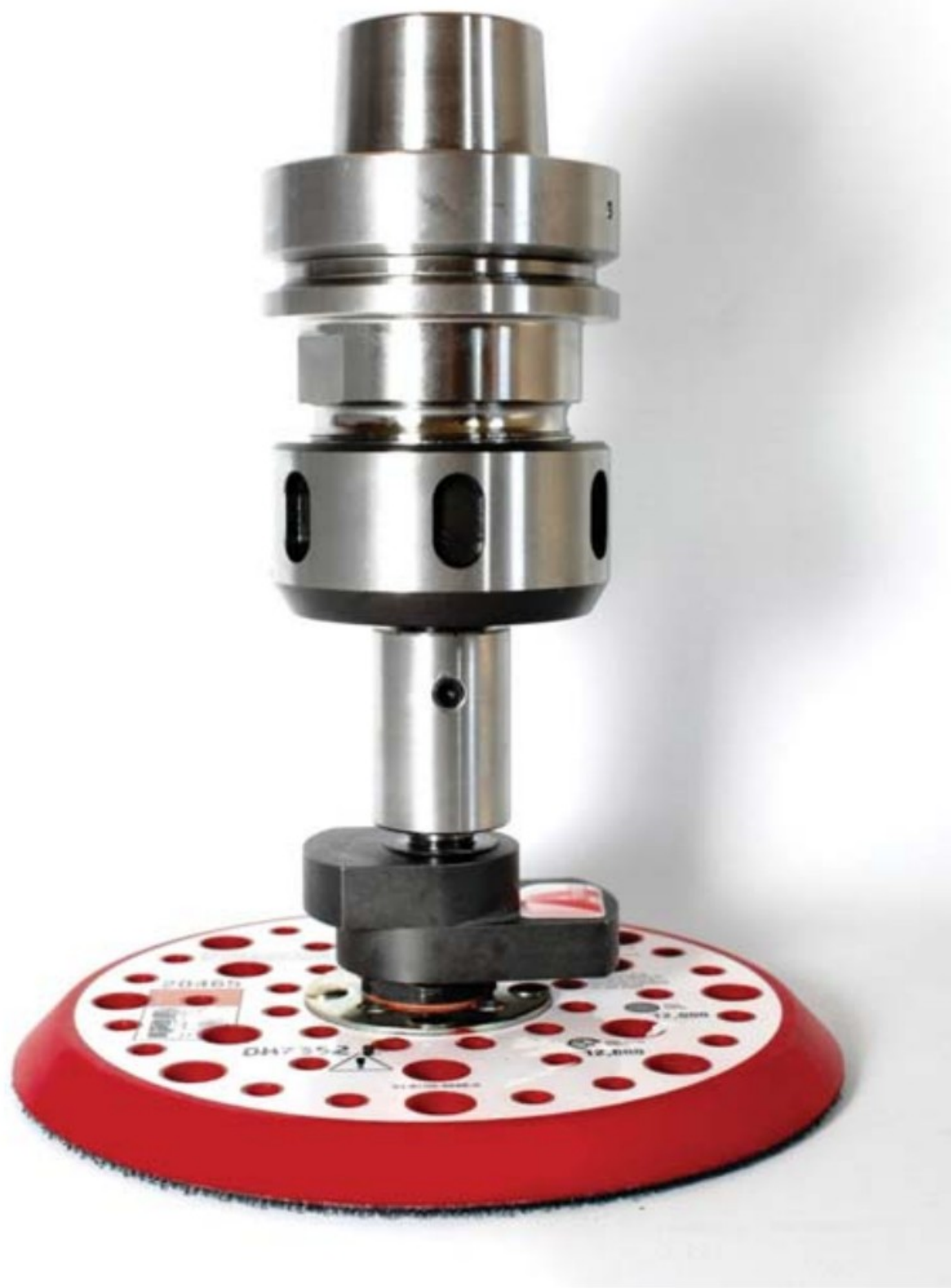
Aggregates can help reduce secondary operations with options like sanding.
