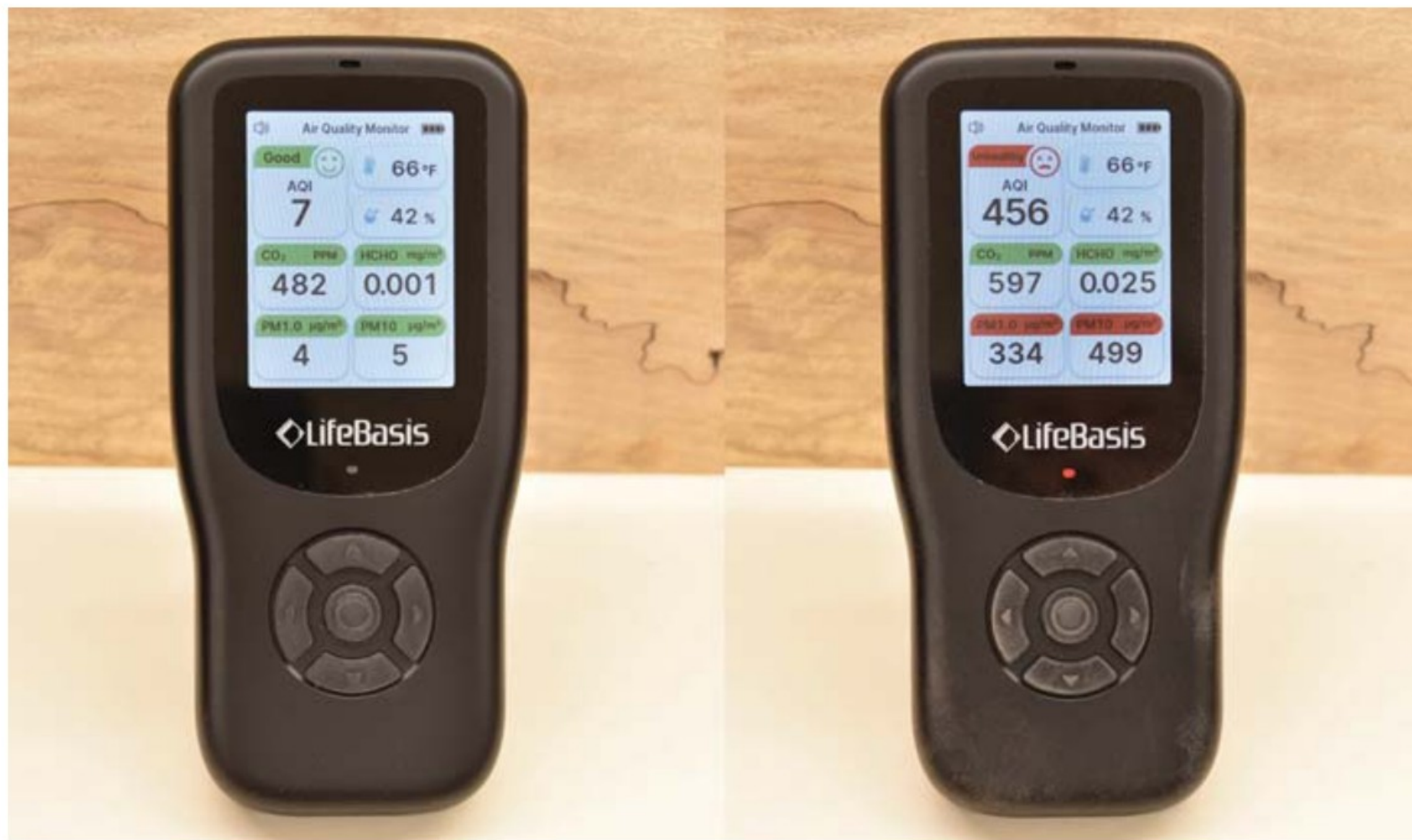
This before/after image shows an air quality meter first reading the air when no tools are running, and then again after using a spindle sander for five minutes with no dust collection.
