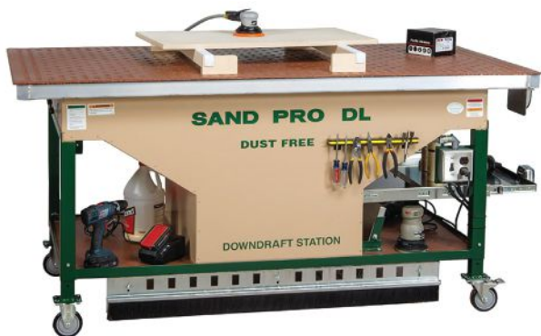
Sandman Products makes sanding tables and booths that capture fine wood dust at its source.
