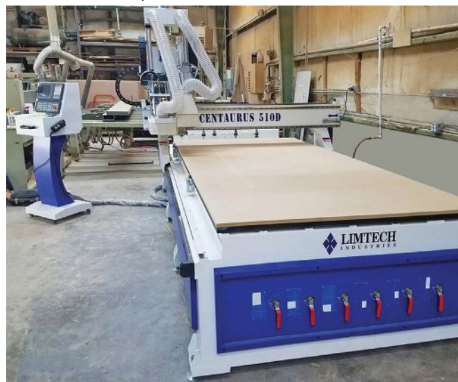
The entry-level industrial series from Limtech, the Centaurus, is designed for nesting and has a linear tool changer.
