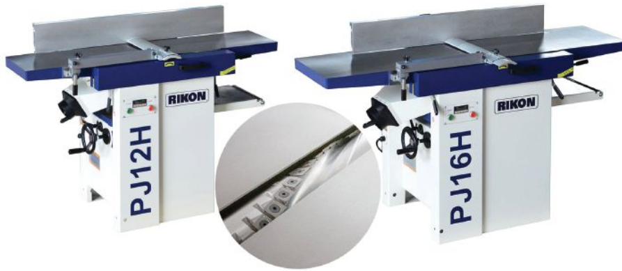
Rikon offers a pair of combination planer/jointers in 12" and 16" options with helical carbide insert cutterheads and DROs.
