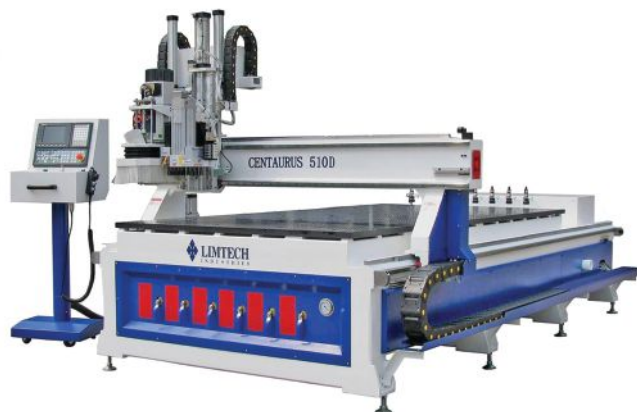
The entry-level CNC from Limtech, the Centaurus, has an eight-position ATC and a 10-hp pump for the vacuum table.
