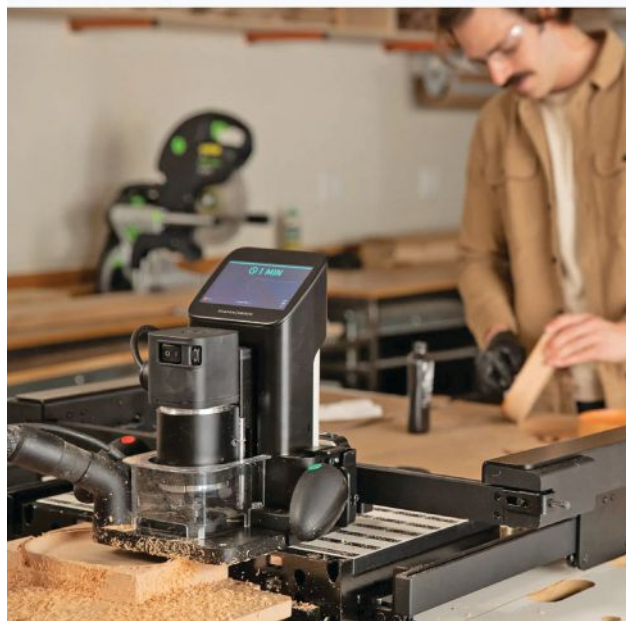
The new BenchPilot from Shaper Tools is a small gantry-like system that transforms the portable CNC into a stationary tool.
