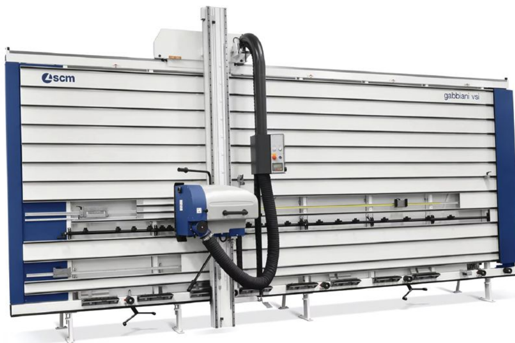
Two Gabbiani panel saws from SCM Group, including the VSi shown, have independent motors for the main and scoring blades.
