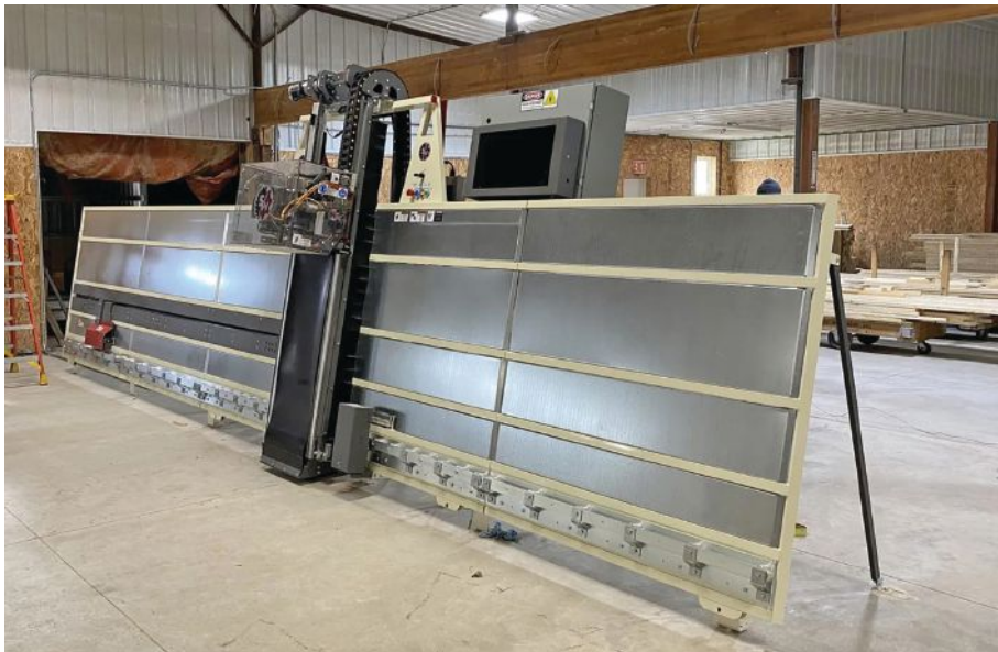
The SpeedWorx saw from Safety Speed Mfg. brings X, Y, Z and C automated controls to a vertical panel saw.
