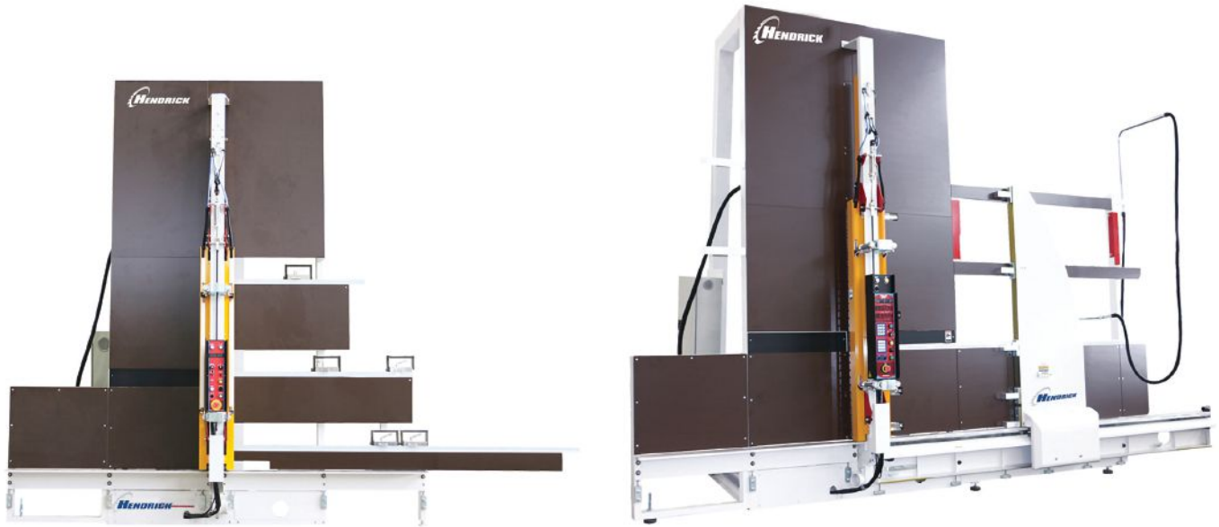
The SPN1 and SPN2 vertical beam saws from Hendrick Mfg. use a full-length pressure beam to hold stacked panels in place.
