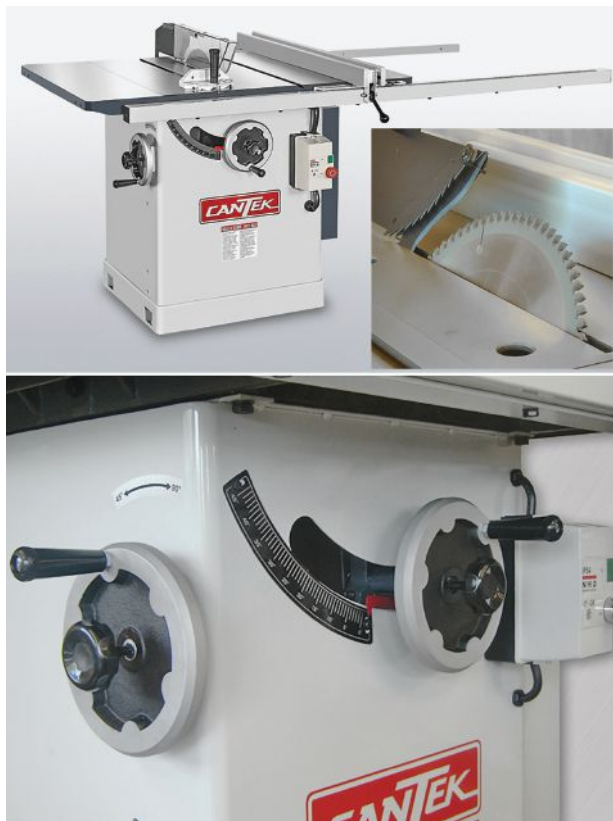
Some woodworkers prefer a right-tilt saw, such as the Cantek TA12, because of scale and splitter alignment issues.
