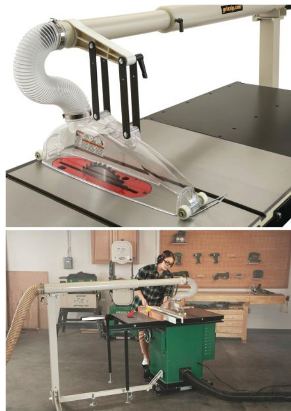
Aftermarket topside dust collection devices, such as Grizzly's T10113 Universal Overarm Blade Guard, can significantly reduce dust.
