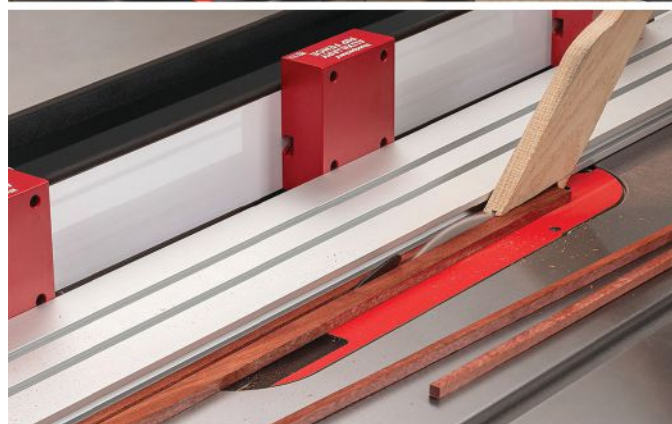
High-low fences, such as this aftermarket Auxiliary Rip Fence from Woodpeckers, can be used to work with thin or tall materials.
