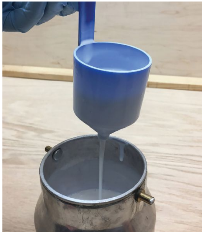
This image from Fuji Spray shows the viscosity of a coating being measured by timing its passage through a measuring cup.
