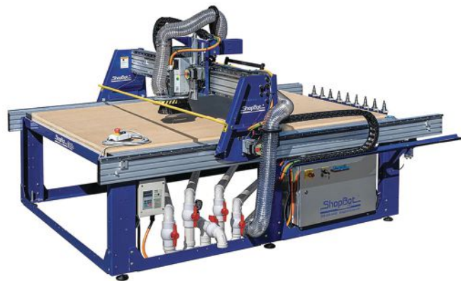
The PRS5 Alpha ATC from ShopBot, available with a 5' x 12' table and an optional fourth axis.
