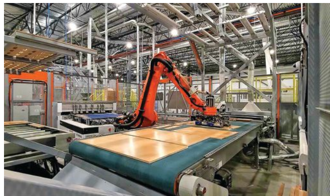
This ARmony robot from Stiles unloads a nested based router, buffers parts, and loads them into a drill and dowel machine.
