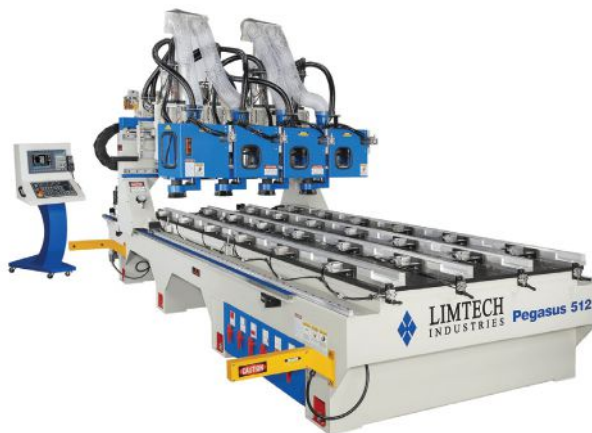
The Pegasus, from Limtech Industries, can be fitted with a 10' x 40' table and eight spindles.
