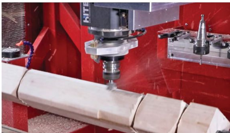
The Legacy Rogue, a fully-enclosed, 5-axis CNC for production turning.
