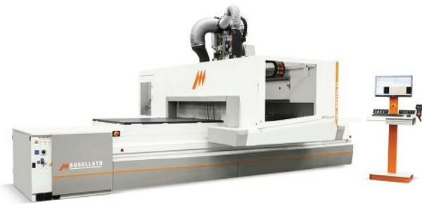
The new Jet Master RTC from Casadei-Busellato, available in 3-, 4- or 5-axis versions and with parts unloading.
