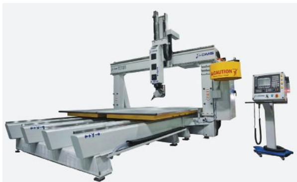
The Teton5 from DMS is a 5-axis machine with a 17.5-hp spindle and pendulum processing.
