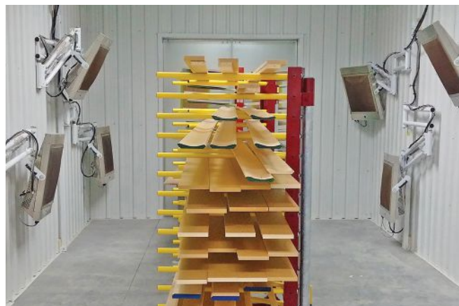
Infrared curing systems, such as the one shown here from Green Fast Cures, reduce contamination and speed up production.
