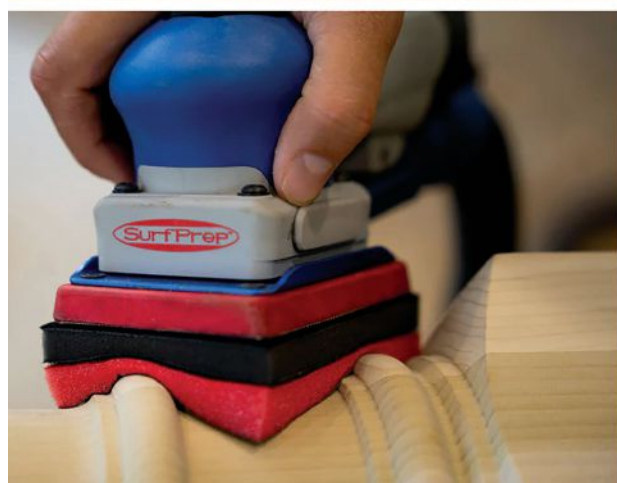
SurfPrep ProFoam pads, new from Total Finishing Supplies, are ideal for knocking down sealer on profiled surfaces.
