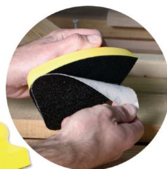
The Gator Zip detail hand sanding kit uses the same refill sandpaper as Black & Decker's Mouse.
