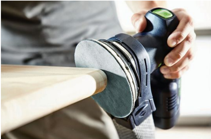
The new Granat Net line from Festool USA reduces dust and increases lifespan with its open net surface.
