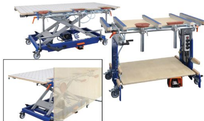
Barth carts from Martin Woodworking allow a woodworker to handle awkward materials by lifting, raising or tilting.
