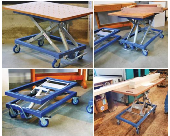
Woodworkers make their own tabletop for the new Rangatge Lift Cart 300, which can lift and move 600 lbs. of material.
