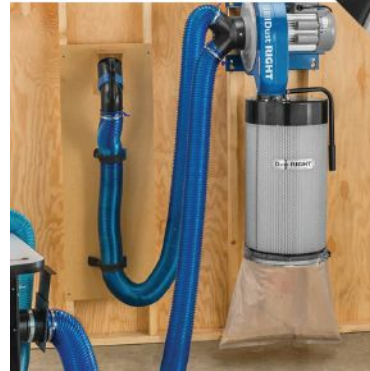
Rockler makes an optional filter for its Dust Right system that places a clear bag below the canister.
