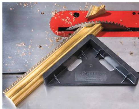
Two fixed value miter cutting guides from Rockler (22-1/2 and 45 degrees) lend accuracy to segmented work.
