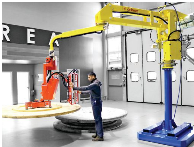
Dalmec's mandrel gripping system for handling and pneumatic tilting of wooden parts.
