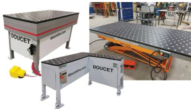
Air tables from Doucet Machineries make it easier to handle large and heavy panels by floating them on a cushion of air.
