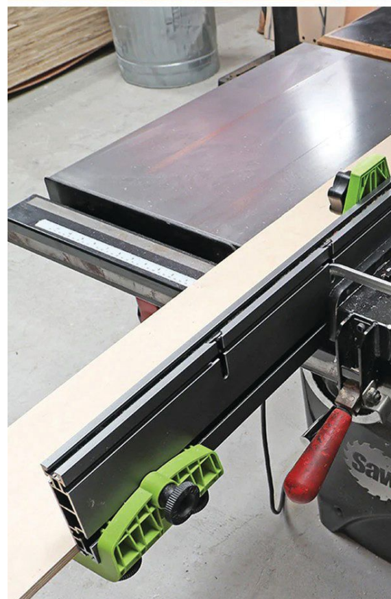
The new Bow Master Tablesaw Pack from Infinity Tools offers infeed, hold-down and feather-board support.
