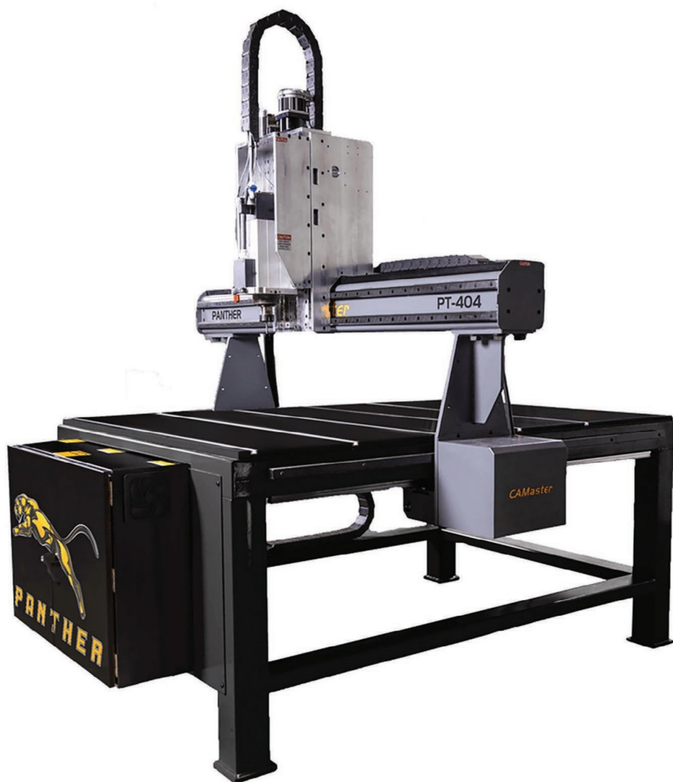
CAMaster makes the 4x4 Panther which comes with a 4.2-hp spindle and WinCNC controls.
