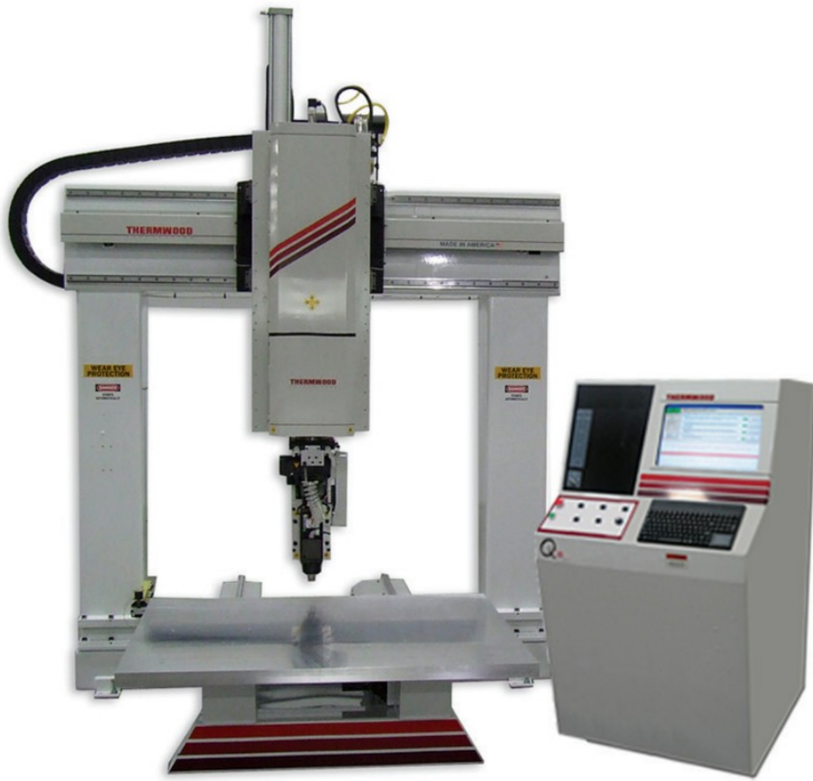
Thermwood's MultiPurpose 67, a 5-axis available with either single or dual moving aluminum tables.
