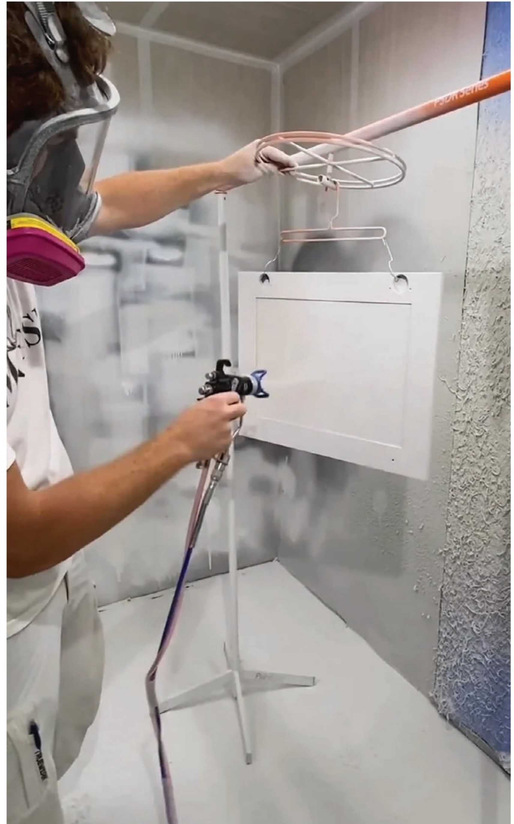
PaintLine's new hinge hooks feature a sharp point to hold doors by their hinge cup holes.
