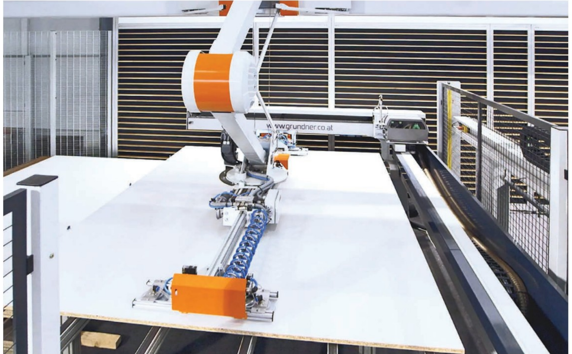
The Store-Master from Holz-Her is built around an automated retrieval-placement arm and can be custom configured.
