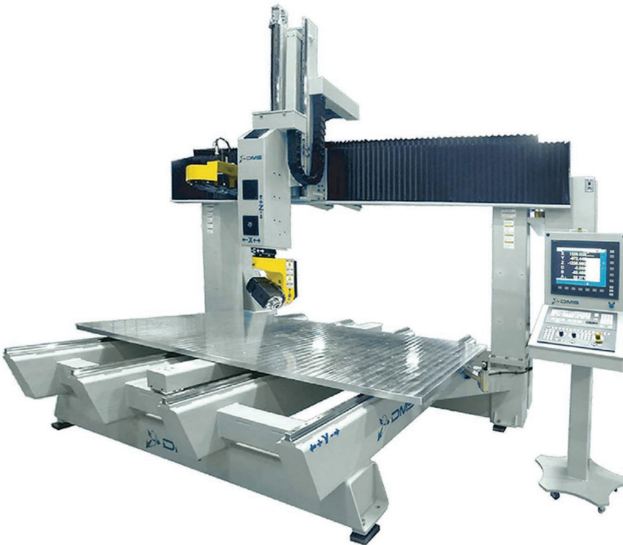
Teton, a 5-axis moving table CNC from DMS, with options for single or twin tables and single or multiple spindles.
