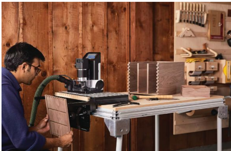
The Shaper Origin and Workbench; making tenons on the Leigh FMT Pro (right).
