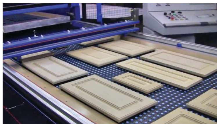
The Thermoformer (top) from Black Bros. and output from the company's larger Thermolaminator machine.
