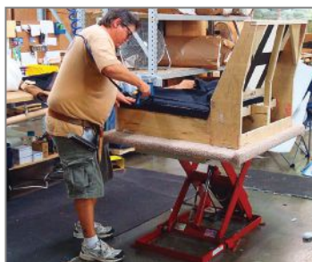
Lift and position workpieces for access to tops and bottoms without bending or reaching.
