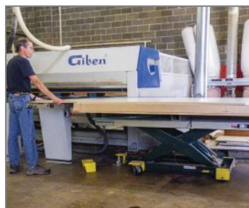
Lift and position panels for easy one person feeding at saws, planes, and CNC routers.
