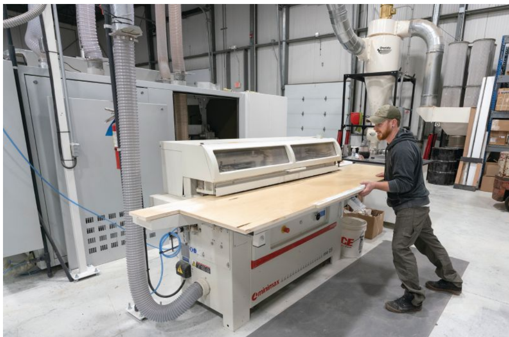
Ron Kilgore (top) on the shop's SCM Minimax me25 edgebander and Tim Criscitello aligning the knives on a toolhead for its Weinig Unimat 218 molder/shaper.
