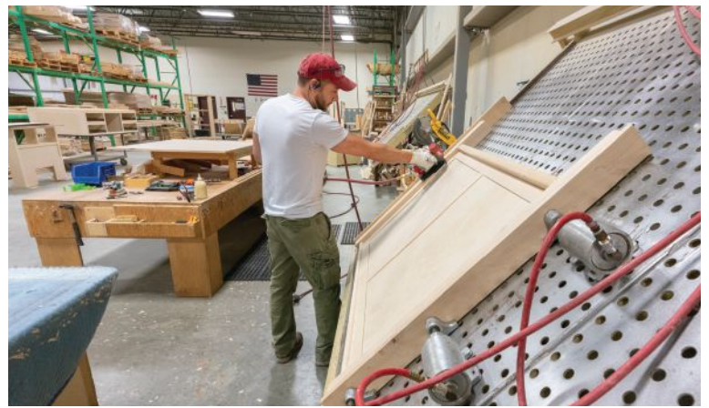
Sean Yeaton (left), the shop's daily production manager, and Antonio Neto assembling a headboard on a Ritter R-250.
