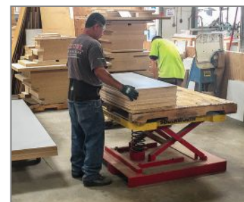
Automatically adjust the height of pallet loads as items are added or removed.
