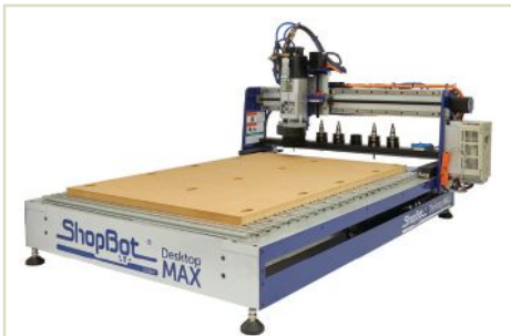
Desktop MAX ATC with Aluminum Deck (general purpose deck) comes standard with an attached MDF spoil board for a wide variety of machining options.
