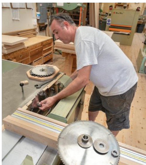
Cressotti (green shirt, top photo) uses the shop's Linmec long bed joiner; Menard (white shirt) changes a saw blade on a SCMI SL12 slider, and a simple solution for storing shaper tooling.
