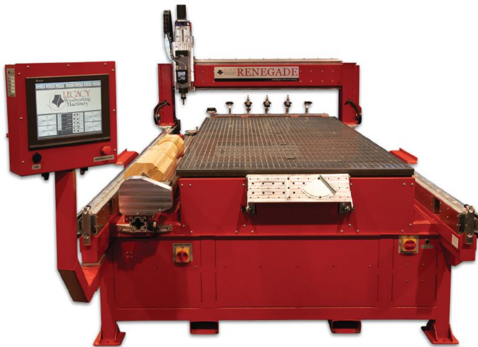
The Renegade features three work stations for panel processing, turning and joinery.
