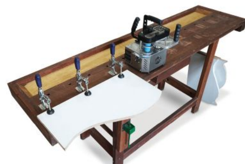
The CBC Flex applies the glue to the substrate.
