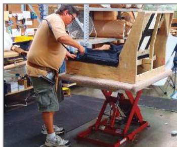
Lift and position workpieces for access to tops and bottoms without bending or reaching.
