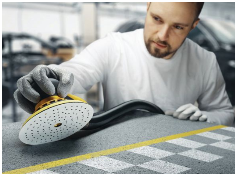
Mirka has introduced film-backed Novastar (left) and paper-backed Iridium abrasives that feature multi-hole patterns for dust extraction.
