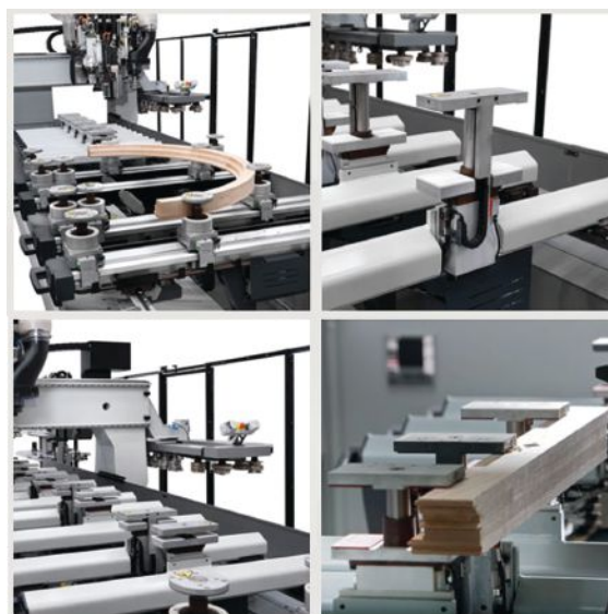
The new Biesse Winline 16 uses an array of work-holding solutions to hold both straight and curved parts, including finger clamps and vacuum modules.
