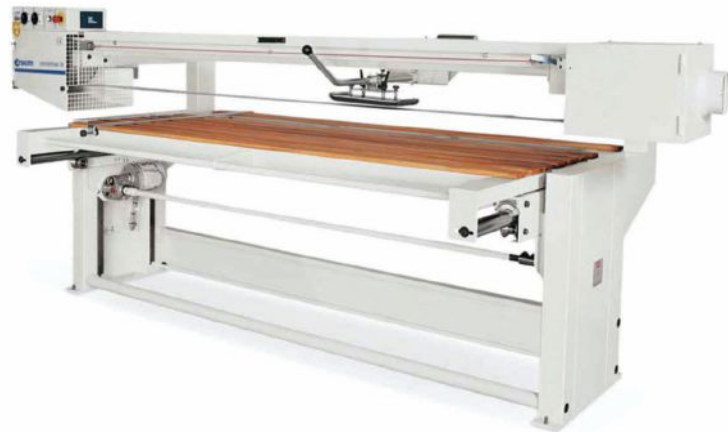
Among the offerings from SCM Group NA is the Minimax Is, a surface belt sander with a double gooseneck and two exhaust hoods.
