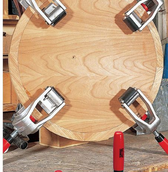
Bessey's edge-gluing clamp that makes quick work of installing solid edgebands.
