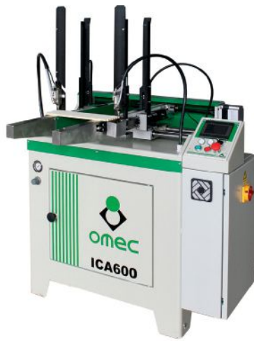
The Omec ICA-600 glue applicator (right) and drawer box clamp.
