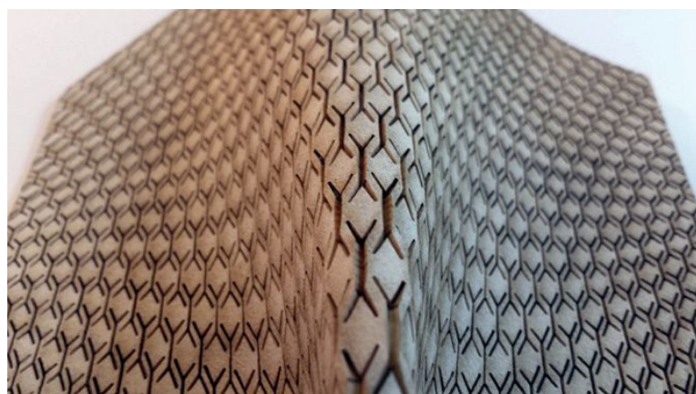
The CNC Shark (above) from Next Wave Automation; examples of lattice cuts made with a laser.
