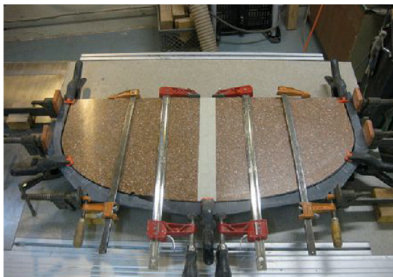
The front foot (above) was made from 14 pieces of solid surface; the top isn't something that could easily be produced with stone.
