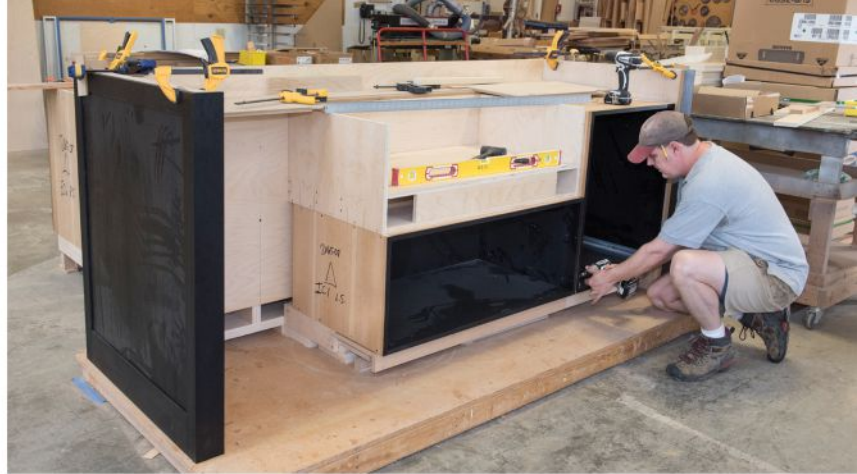
Bruton Strange installs drawer slides in a cabinet.
