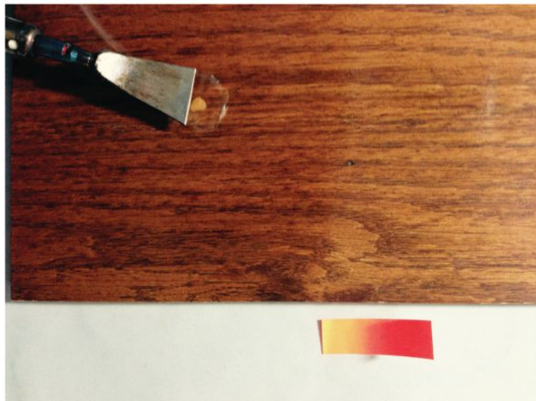
A burn-in knife should be held at an angle of 30 degrees or less.
