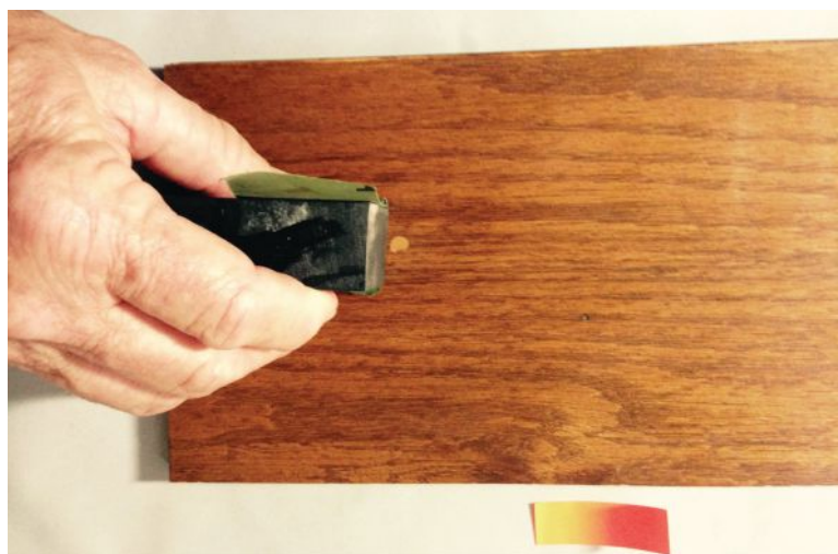
Sand with 400A wet or dry paper to complete the leveling process.
