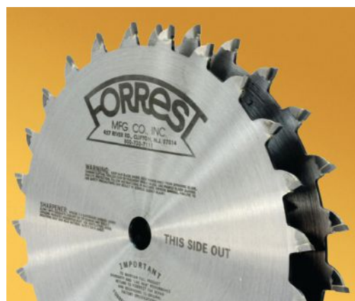
Among Forrest Manufacturing's new blades is this 8" diameter thin kerf dado set (DK0824316) that was designed for clean-cutting 3/16" wide grooves.
