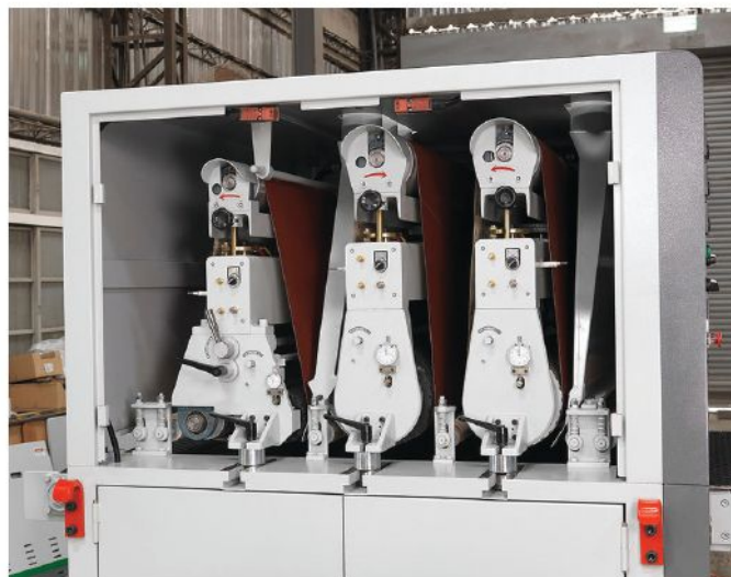
The Ironwood S124RK (left) and S134RRK showing its three sander heads.
