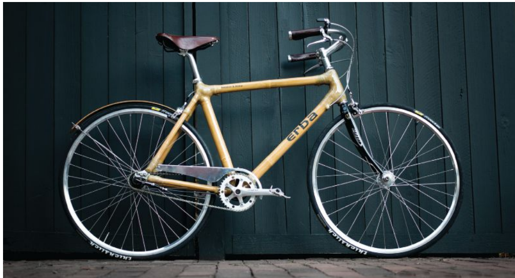
The "Erban" bicycle at Messler, made with bamboo and hemp.
