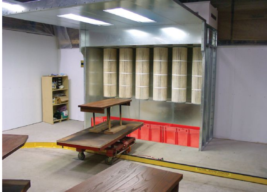
Servair's sanding booths clean the air and return it to the shop.
