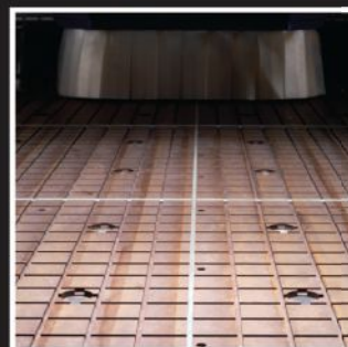
Nesting table 6 vacuumfields on phenolic table
