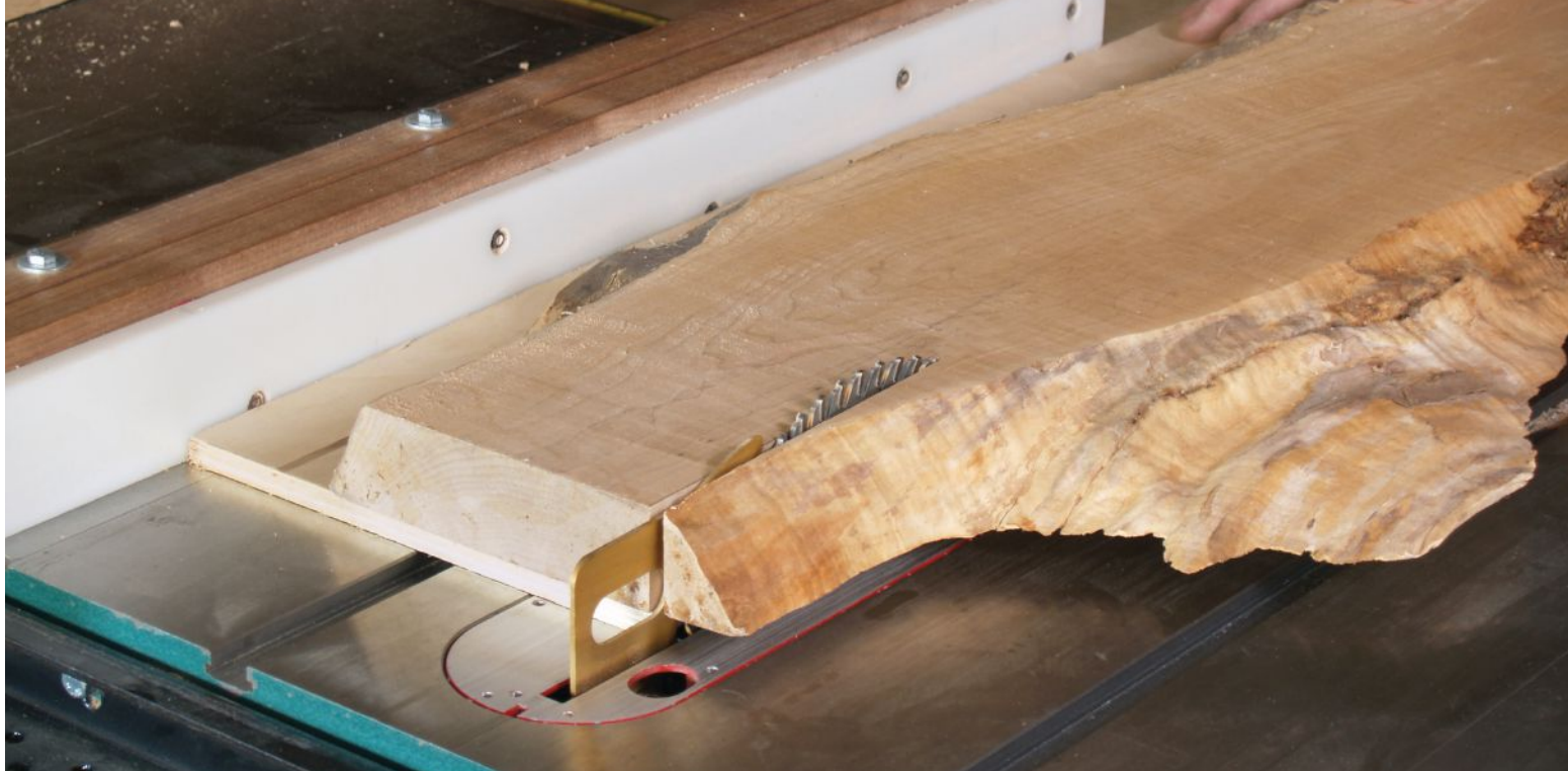
Getting a straight cut without a straight edge is a problem. An easy solution is to attach a plywood base.
