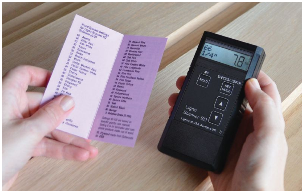
A wood species chart is available with most meters. When using any meter, corrections for species should be done to get the right moisture values.
